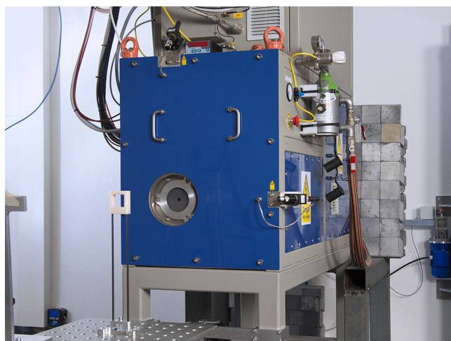
FIG. 12. The Oriatron/eRT6 (PMB-Alcen) is currently considered the reference for demonstrating and investigating the FLASH effect, as more than 15 peer-reviewed publications produced with the Oriatron eRT6 have reproduced the FLASH effect in many organs and animal models.
