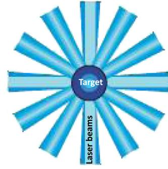
FIG. 23. Schematic of laser-direct-drive ICF. Multiple laser beams symmetrically illuminate a spherical shell containing DT fuel.
