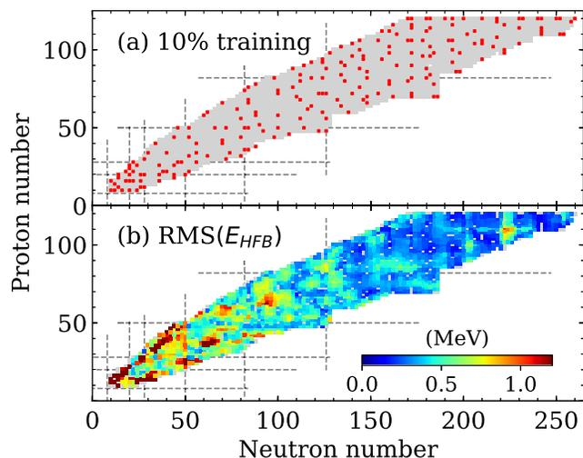
FIG. 3. DFT emulator with ANNs. (a) Database nuclei (gray region) as a function of  $N$  and  $Z$ . Nuclei included in the 10% training dataset obtained by active learning are marked as dots. (b) Root mean square deviation between the total energy for the testing dataset calculated in DFT ( $E_{HFB}$ ) and with the committee of ANNs. Adapted from Lasserri *et al.*, 2020.
