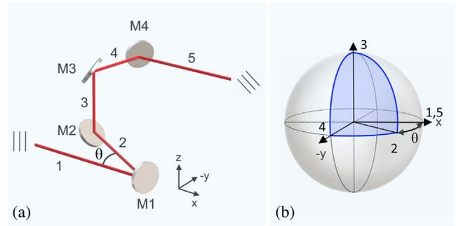
FIG. 7. Generation of SR phases. (a) Linearly polarized beam taken along a nonplanar trajectory. The mirrors M2 and M3 form a beam elevator. At the end of the trajectory, the polarization axis is rotated. (b) Path formed on the sphere of the spin directions.
