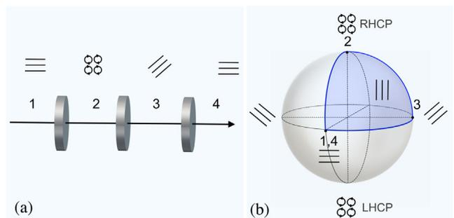
FIG. 2. Sequence of polarization transformations. (a) Practical realization. (b) Geometric interpretation: a closed path is traced on the Poincaré sphere.
