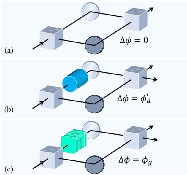
FIG. 1. Phase measurements with Mach-Zehnder interferometers. (a) Balanced interferometer with arms of equal optical path length. (b) Introducing a dynamic phase by changing the optical path length with a piece of glass in one arm. (c) Introducing a geometric phase by performing a succession of state transformations in one arm.
