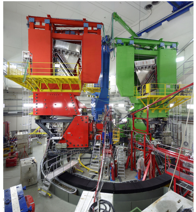
FIG. 12. Top image: schematics of the three-spectrometer setup of the A1 experiment at Mainz. From Blomqvist et al. , 1998. Bottom: photo showing spectrometers A, B, and C in red, blue, and green, respectively. The electron beam progresses from right to left. From Weis, 2003.
