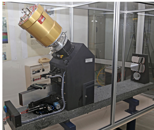
FIG. 1. ELODIE spectrograph on display at OHP. On the left we see the échelle grating with the grooves facing us. On the left side, the optical fibers feeding the spectrograph are clearly visible (in orange). On the top sits the cryostat with inside the CCD detector. The “cross-dispersing” optic (not visible) is located in the vertical dark painted holding structure.
