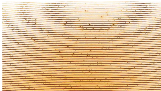
FIG. 2. Middle cut of ELODIE image of a stellar spectra observed with simultaneous thorium recorded on the CCD. One clearly distinguishes the curved spectroscopic order of the stellar spectra from the interlaced emission spectrum due to simultaneous thorium lamp illuminating the second fiber.
