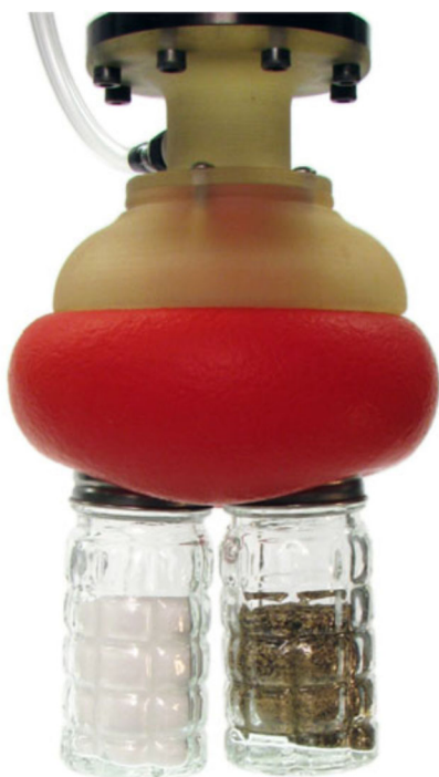
FIG. 9. Universal grippers based on jamming in granular material. A rubber membrane, containing a granular material, can be deformed so that its shape conforms to that of an object to be manipulated. The membrane can be evacuated so that the granular material becomes rigid due to the external air pressure. This produces a universal gripper that can lift a large variety of objects with different shapes. Here the gripper is shown picking up salt and pepper shakers. From Amend et al. , 2012 .
