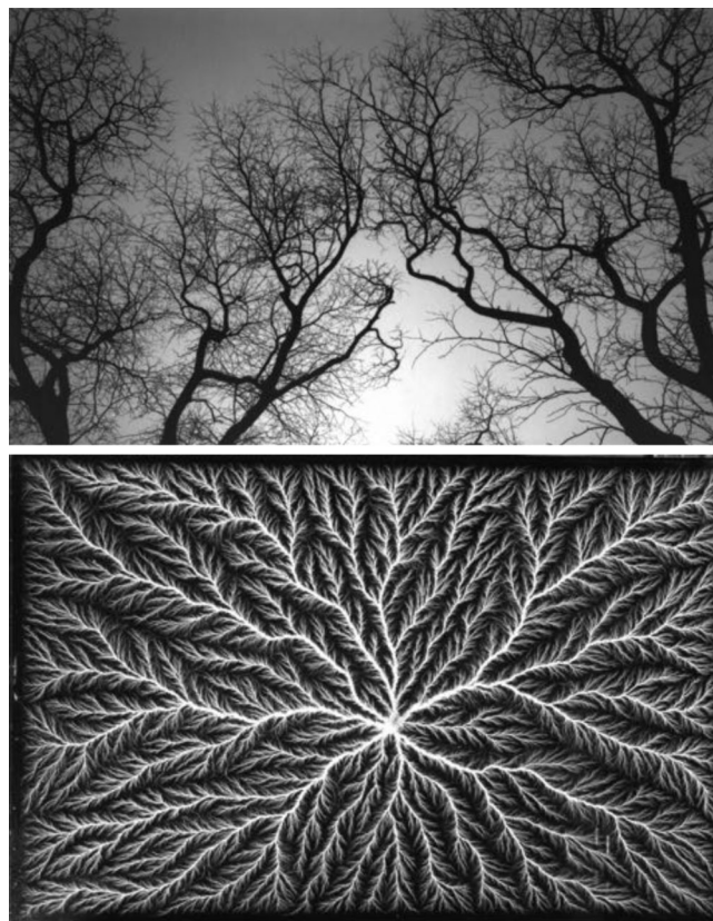
FIG. 3. (Top) Branching patterns seen in the limbs of trees and (bottom) in dielectric breakdown of a Lichtenberg figure.
