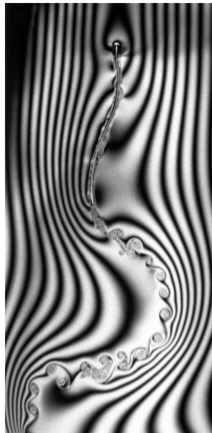
FIG. 1. The oscillatory flapping state of a filament in a flowing two-dimensional soap film. Flow structures, modulated by the moving filament, are advected downstream. The flow is visualized using interference imaging. From Zhang et al. , 2000.
