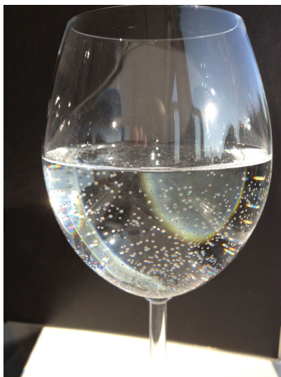
FIG. 41 (color online). Glass filled with cold tap water (which is air oversaturated) after 24 h under room temperature conditions: Many surface bubbles have nucleated and survived.
