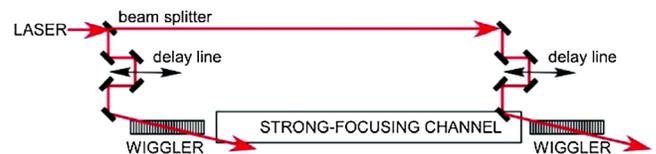
FIG. 43 (color online). A schematic of the laser-assisted conditioner. From Zholents, 2005a.
