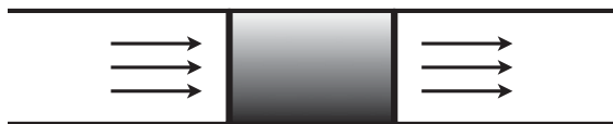
FIG. 2. Schematic of an experiment measuring mass flow through a supersolid. Superfluid liquid flows across the central section filled with supersolid, of the same substance. The setup as shown can work only at the melting pressure. In the case of ^4\text{He} , modifications involving Vycor segments and temperature gradients allow one to extend measurements to higher pressures. From Ray and Hallock, 2008.
