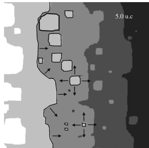
FIG. 17. Simulated surface morphology after five unit-cell layers on substrates with a vicinal angle of 0.6°. The advancing steps, indicated by the solid lines, coalesce with the growing islands on the terraces. In this simulation, the deposition temperature was set to 600 °C, E_S = 0.75 eV, and E_N = 0.6 eV, the pulse repetition rate = 2 Hz, and the number of pulses needed for completion of one unit-cell layer is 20.
