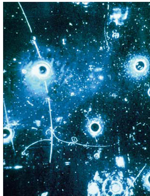
FIG. 4 (color online). The first candidate leptonic neutral-current event from the Gargamelle CERN experiment. An incoming muon-antineutrino knocks an electron forwards (towards the left), creating a characteristic electronic shower with electron-positron pairs. Photograph from CERN.
