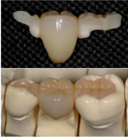
FIG. 62. (Color online) This dental bridge is made from a fiber-reinforced composite with braided fibers made from polyethylene. Due to the braided structure, this composite is four times tougher than a composite made from the same materials but without the braiding (Karbhari and Strassler, 2007). Courtesy of H. Strassler, University of Maryland Dental School and V. Karbhari, University of Alabama, Huntsville.
