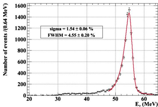
FIG. 73. (Color online) Energy spectrum for 55 MeV gamma rays measured with the large MEG prototype (Baldini *et al.*, 2005).
