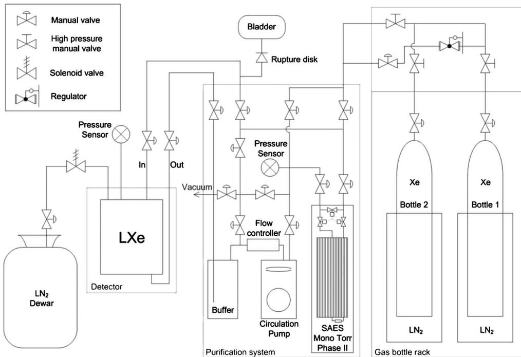
FIG. 55. The XENON10 detector purification system (Aprile *et al.*, 2010).
