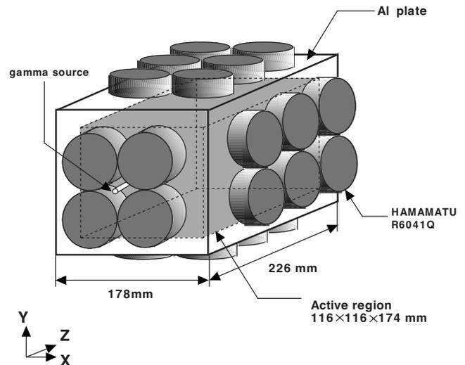
FIG. 37. Schematic of the LXe scintillation prototype with  $32 \times 2$  in. PMTs (Hamamatsu R6041Q) developed for the MEG experiment (Mihara et al., 2002).
