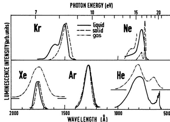
FIG. 18. Emission bands in liquid rare gases, together with solid- and gas-phase spectra (Jortner *et al.*, 1965; Schwenter, Kock, and Jortner, 1985).
