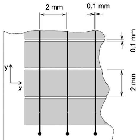
FIG. 78. The ministrip plate of the Coimbra PET prototype (Solovov *et al.*, 2002a).
