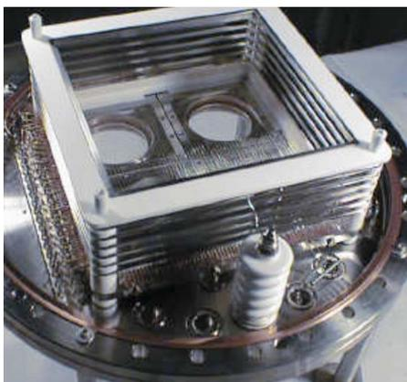
FIG. 49. (Color online) Photo of the LXeGRIT TPC structure (cathode removed) (Aprile *et al.*, 2004b).
