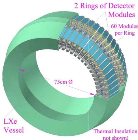
FIG. 80. (Color online) Schematic of the Columbia full scale LXe Compton PET (Giboni *et al.*, 2007).
