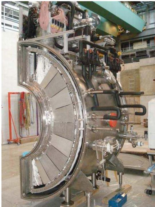
FIG. 74. (Color online) Photo of the full scale MEG LXe scintillation calorimeter.
