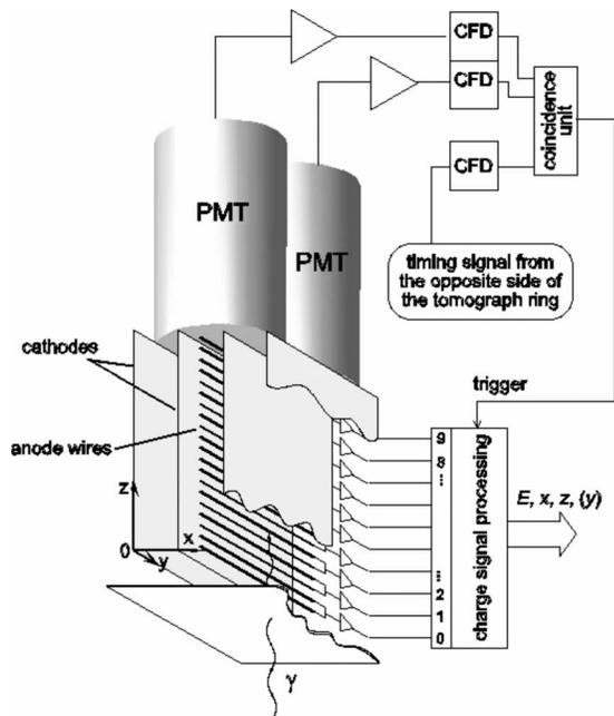
FIG. 77. Schematic of the Coimbra PET prototype (Chepel *et al.*, 2001).
