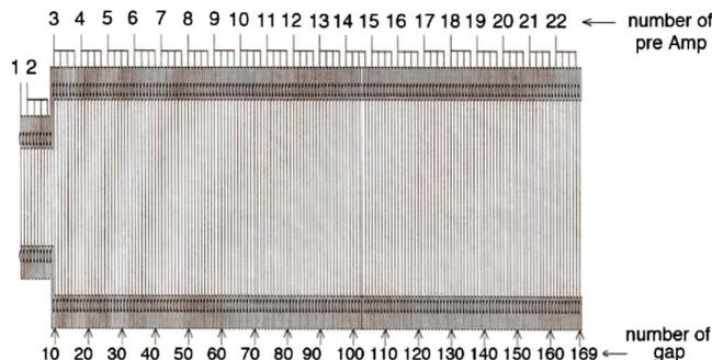
FIG. 67. (Color online) Schematic of the Waseda multiplate LXe ionization calorimeter (Okada *et al.*, 2000).
