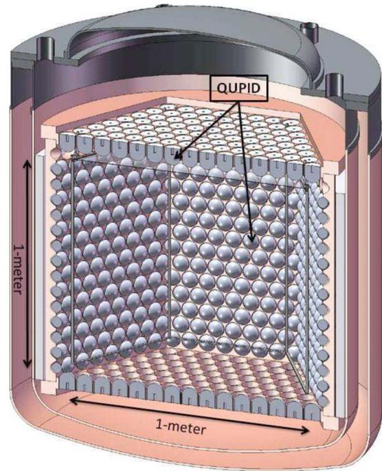
FIG. 59. (Color online) Schematic of the XENON1T detector.
