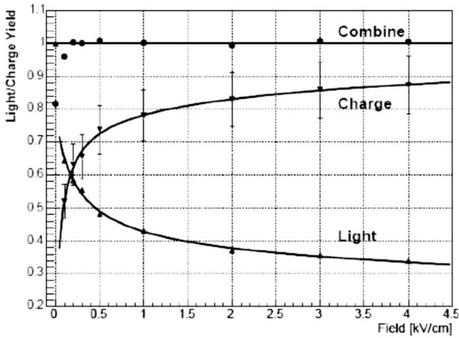
FIG. 40. Light and charge as a function of drift field for  $^{137}\text{Cs}$  662 keV  $\gamma$  rays (Aprile *et al.*, 2007b).
