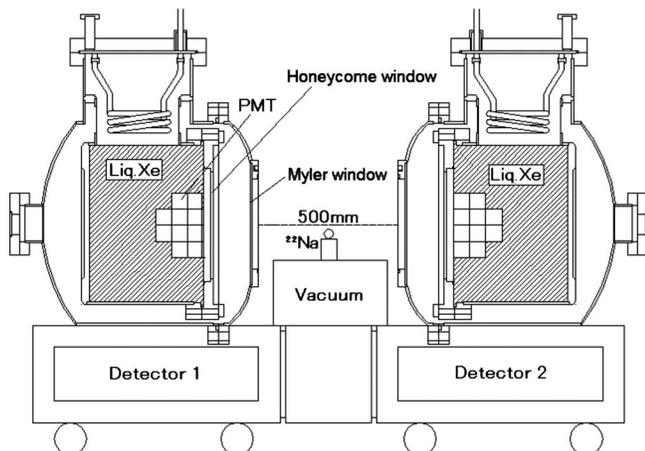
FIG. 83. Schematic of the Waseda TOF PET prototype (Nishikido *et al.*, 2004).
