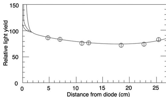
FIG. 69. Relative light yield as a function of the distance from the Si photodiode, measured with cosmic-ray muons. Monte Carlo curves are shown for different light collimators (Chen *et al.*, 1993).
