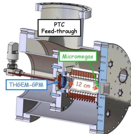
FIG. 81. (Color online) Schematic of the Nantes LXe Compton PET prototype (Grignon *et al.*, 2007).
