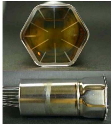
FIG. 64. (Color online) Photo of the hexagonal PMT of the XMASS detector.
