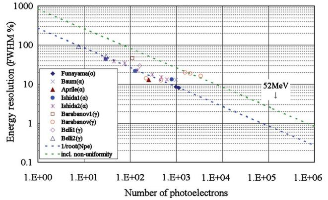
FIG. 36. (Color online) Relation between energy resolutions and the estimated number of photoelectrons obtained for  $\alpha$  particles and  $\gamma$  rays (Doke and Masuda, 1999, and references therein). The lower line expresses a relation of energy resolution which is inversely proportional to the square root of the number of photoelectrons. The upper line shows a worse energy resolution expected from the nonuniformity of light collection.
