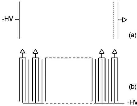
FIG. 35. Schematic of electrodes arrangement for an ionization calorimeter. (a) Gridded ionization chamber with a long sensitive region. (b) Multiparallel plate electrode system (Doke, 1993).
