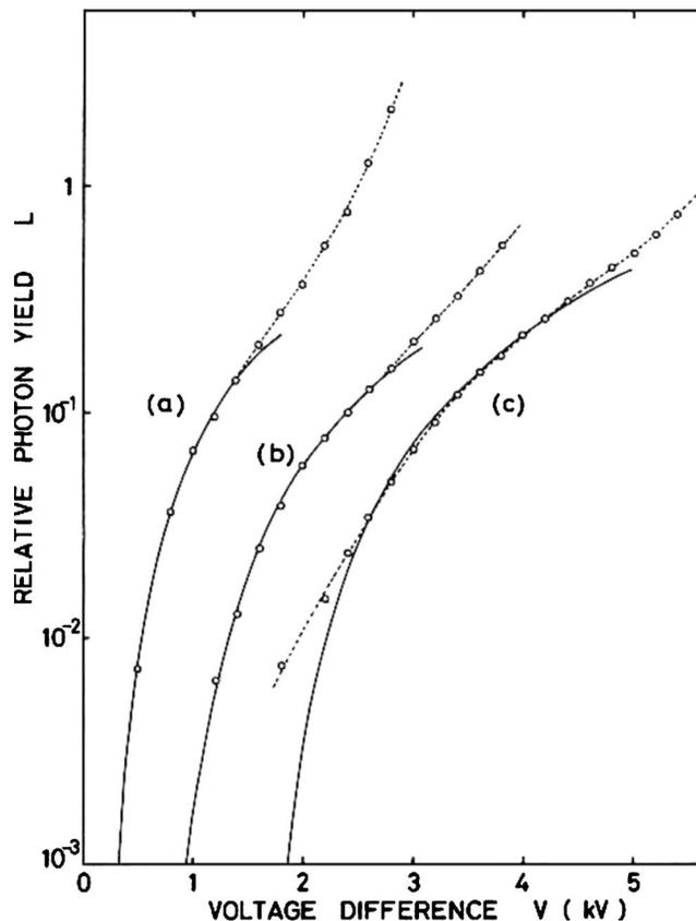
FIG. 14. Relative photon yield of proportional scintillation and charge gain as a function of applied voltage to anode wires of different diameter. Solid lines are results of the fit by Derenzo *et al.* (1974) to the data points in the region of the ionization chamber mode: (a) for 4- $\mu\text{m}$ -diameter wire, (b) for 10  $\mu\text{m}$ , and (c) for 20  $\mu\text{m}$  (Masuda *et al.*, 1979).
