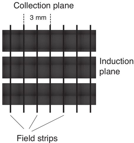
FIG. 32. An example of two-dimensional position-sensitive electrode, with orthogonal strips for collection and induction signals (Cennini *et al.*, 1994).
