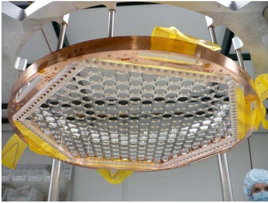
FIG. 76. (Color online) Photo of one EXO-200 anode plane. Induction and charge collection grids cross at  $120^\circ$ . The LAAPD support platter is visible behind the grids (Gratta, 2009).
