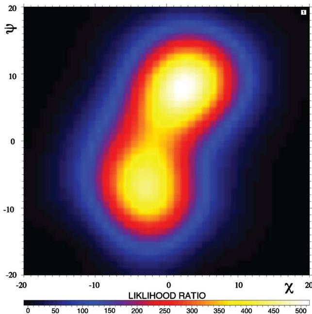
FIG. 51. (Color online) LXeGRIT image (reconstructed angles in degrees) of two calibration sources,  $^{60}\text{Co}$  and  $^{60}\text{Na}$ , using a maximum likelihood imaging technique (Aprile *et al.*, 2008).
