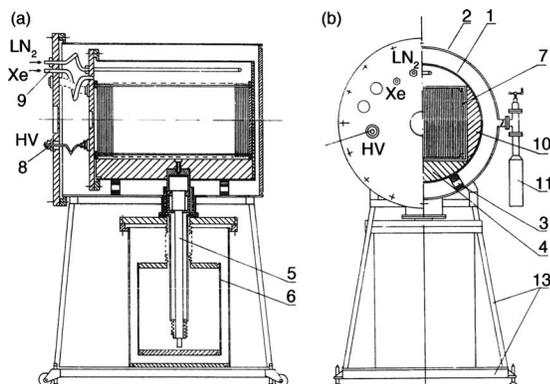
FIG. 65. Schematic of the Russian LXe ionization calorimeter. (a) and (b) Inner (1) and outer (2) cylindrical vessel, (3) multiplate supports, (4) and (10) aluminum segments, (5) copper bar, (6) cryostat with LN<sub>2</sub>, (7) electrode system, (8) HV connector, (9) Xe gas supply tube, (11) zeolite trap (Baranov *et al.*, 1990).
