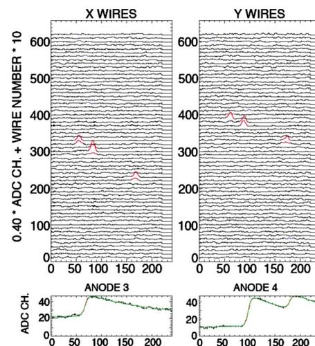
FIG. 43. (Color online) Display of a 1.8 MeV  $\gamma$ -ray event with multiple Compton interactions, recorded with the LXe-TPC (Aprile *et al.*, 1998).
