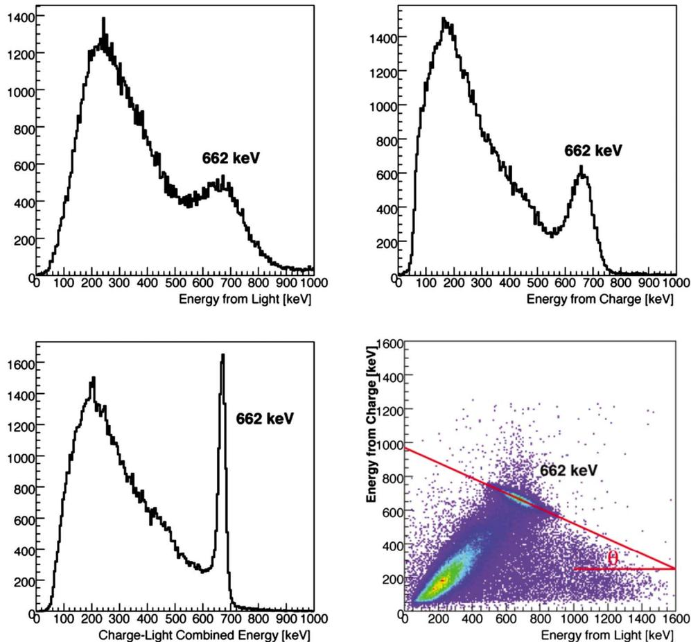
FIG. 41. (Color online) Energy spectra of  $^{137}\text{Cs}$  662 keV  $\gamma$  rays measured with 1 kV/cm field in LXe, separately from charge and light (top panels) and from combined charge and light (lower panel, left); charge-light anticorrelation and its angle (lower panel, right) (Aprile *et al.*, 2007b).
