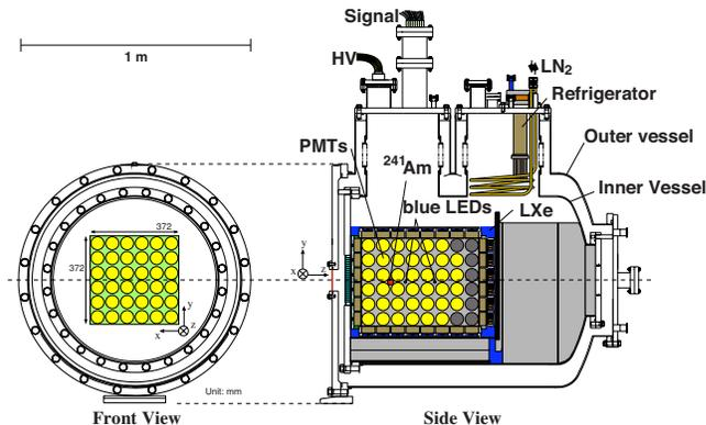
FIG. 72. (Color online) Schematic of the large MEG prototype (Mihara, 2004).
