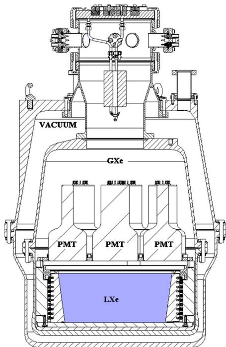
FIG. 60. (Color online) Schematic of the ZEPLIN II detector (Alner *et al.*, 2007).
