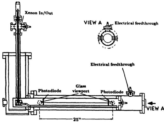
FIG. 68. Schematic of a full length liquid xenon cell for light collection uniformity tests (Chen *et al.*, 1993).
