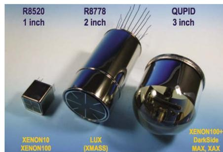
FIG. 53. (Color online) Photo of the different Hamamatsu PMTs developed for the XENON and XMASS dark matter experiments.
