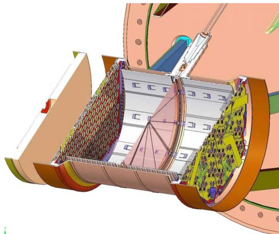
FIG. 75. (Color online) Schematic of the EXO-200 TPC (Gratta, 2009). The length of the TPC as well as the diameter of the TPC planes are 40 cm.
