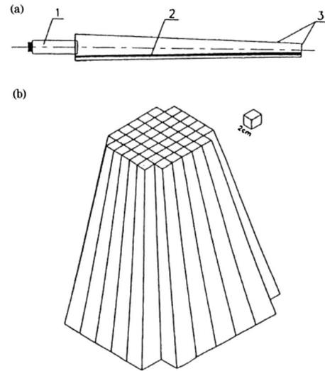
FIG. 70. Schematic of the MIT-ITEP-Dubna LXe scintillation calorimeter. (a) Unit cell of the calorimeter: 1, PMT; 2, fragment of p-terphenyl strip; 3, Mylar reflector. (b) Assembly of the full calorimeter reflector structure (Akimov *et al.*, 1995).
