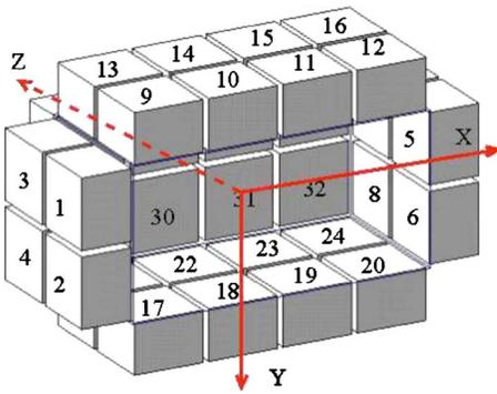
FIG. 82. (Color online) Arrangement of 32 PMTs in Waseda TOF PET prototype (Nishikido *et al.*, 2004).
