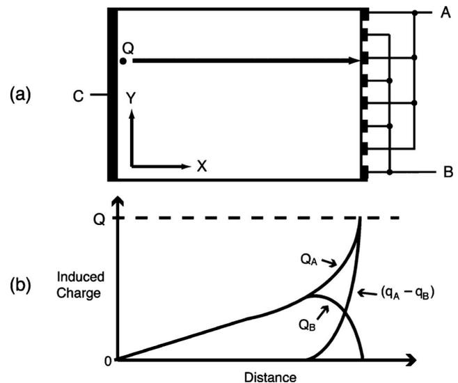
FIG. 31. Schematic of an ionization chamber with coplanar electrodes. (a) Anode made of parallel strips. (b) Time variation of the induced charge signals and the resulting signal in case the charge  $Q$  is collected onto the group of strips marked as  $A$  (Luke, 1995).
