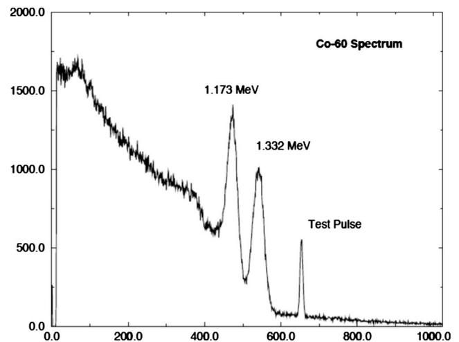
FIG. 34. The energy spectrum of  $^{60}\text{Co}$  gamma rays measured with the gridded ionization chamber shown in Fig. 30 at 4 kV/cm drift field (Aprile *et al.*, 2002). The energy resolution of the 1.3 MeV line is about 5% (FWHM).
