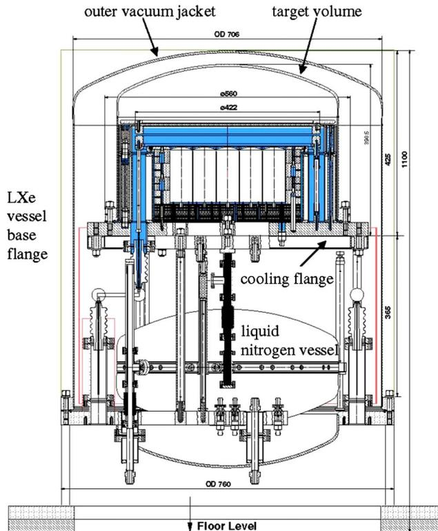
FIG. 61. (Color online) Schematic of the ZEPLIN III detector (Lebedenko, 2008).
