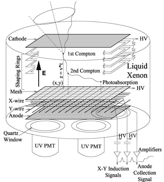
FIG. 47. Schematic of a LXe-TPC as Compton telescope (Aprile *et al.*, 2004b).
