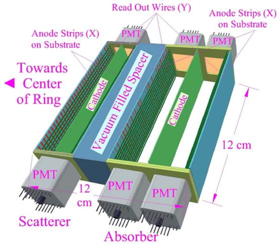
FIG. 79. (Color online) Schematic of the Columbia LXe Compton PET unit cell (Giboni *et al.*, 2007).
