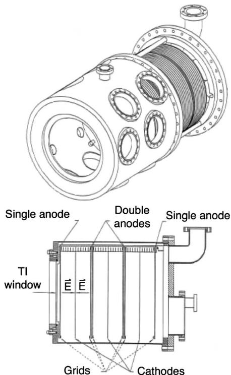
FIG. 71. Schematic of the RAPID LXeTPC. TPC vessel with Ti window for incident  $\gamma$  rays and quartz windows for PMTs (top) Cross section of the electrodes for charge readout (bottom) (Bressi *et al.*, 1998).
