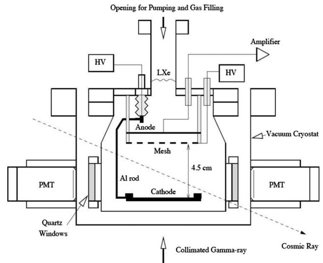
FIG. 30. Schematic of a 3.5 l LXe gridded ionization chamber, triggered by the scintillation light (Aprile *et al.*, 2002).
