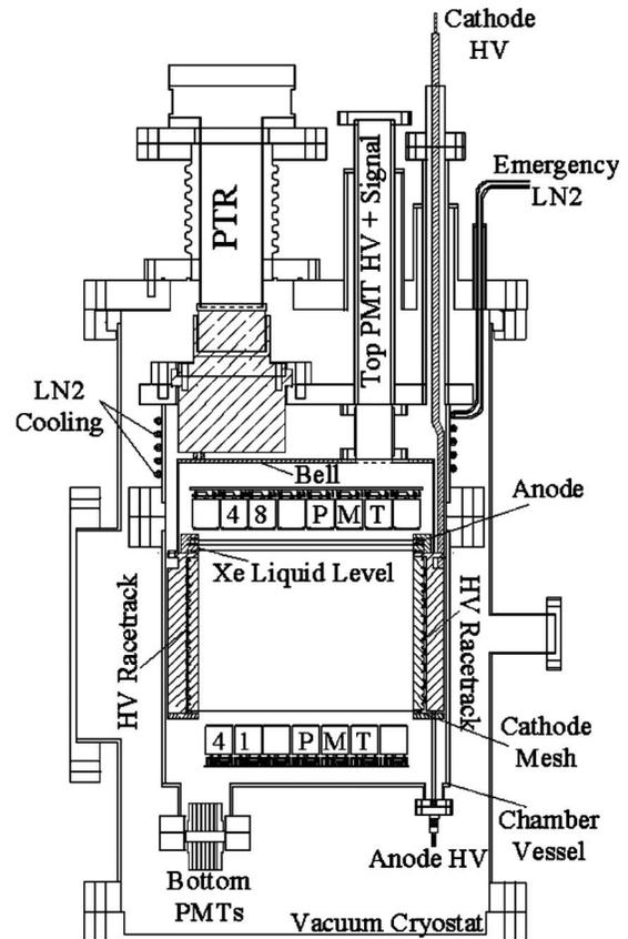
FIG. 54. Schematic of the XENON10 detector (Aprile *et al.*, 2010).
