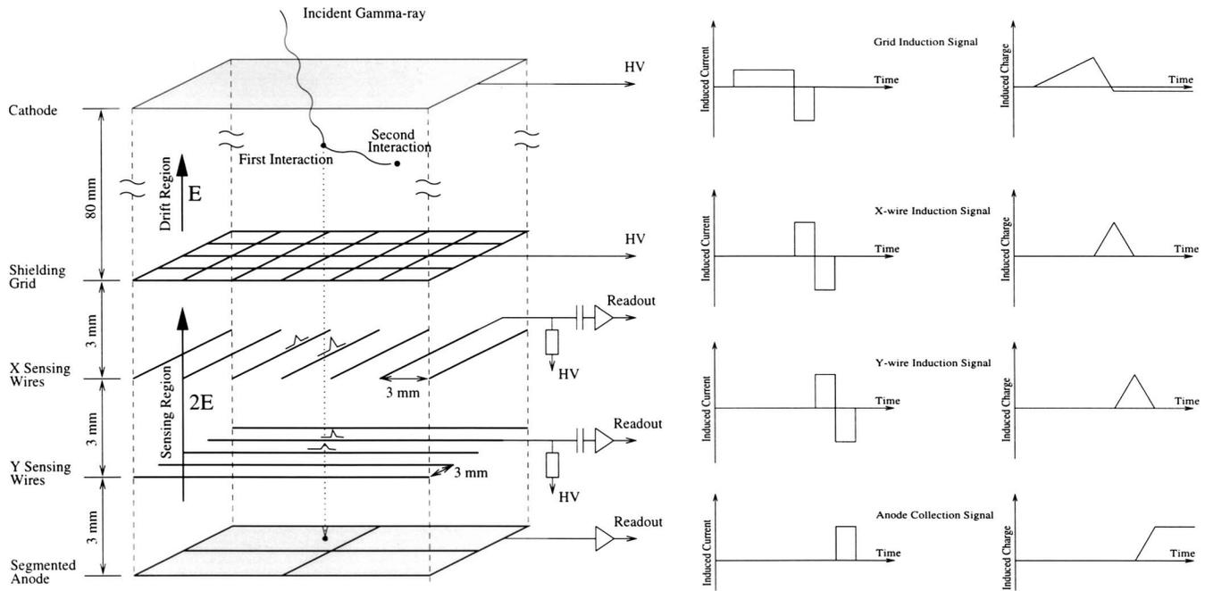
FIG. 42. Schematic of the LXe-TPC. Left: Electrodes structure (not to scale). Right: Corresponding pulse shapes (Aprile *et al.*, 1998).
