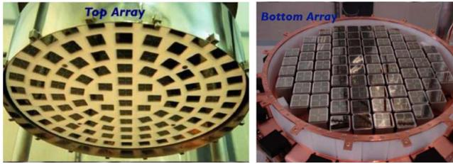
FIG. 57. (Color online) Photos of the top and bottom PMT arrays of the XENON100 detector.
