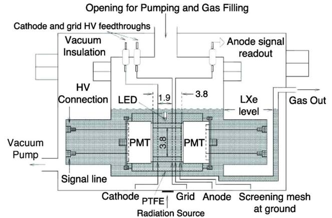
FIG. 39. (Color online) Schematic of a “sum signal mode” detector (Aprile *et al.*, 2007b).
