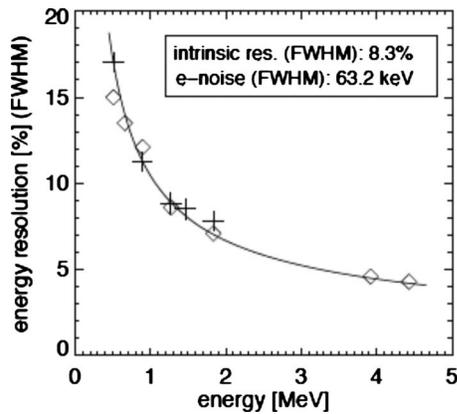
FIG. 50. The energy resolution of LXeGRIT as a function of energy, as measured in flight. The crosses and diamonds are data from two balloon flights (Curioni *et al.*, 2007).
