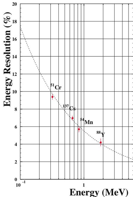
FIG. 38. (Color online) Energy resolution ( $1\sigma$ ) as a function of gamma-ray energy, measured with the MEG detector. The data follow  $1/\sqrt{N_{\text{phe}}}$  as expected (Mihara *et al.*, 2002).
