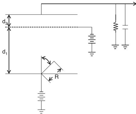
FIG. 29. Schematic of a gridded ionization chamber.  $d_1$  is the drift gap between the cathode (on the bottom) and the Frish grid,  $d_2$  is the field region between the Frish grid and the anode (on the top).
