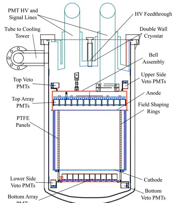
FIG. 56. (Color online) Schematic of the XENON100 detector (Aprile and Baudis, 2008).
