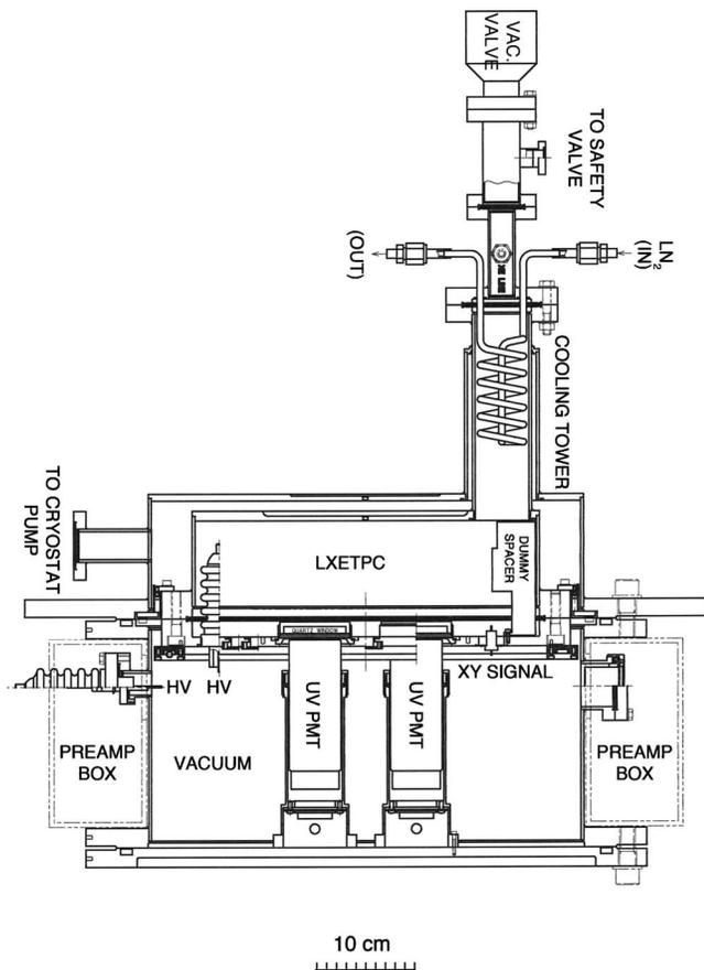
FIG. 48. Mechanical drawing of the LXeGRIT TPC (Aprile *et al.*, 2004b).
