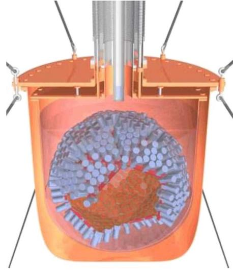
FIG. 63. (Color online) Schematic of the XMASS detector (Suzuki, 2008).
