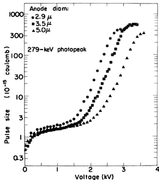
FIG. 13. Pulse height of 279 keV photopeak as a function of voltage for 2.9-, 3.5-, and 5.0- $\mu\text{m}$ -diameter anode wires (Derenzo *et al.*, 1974).
