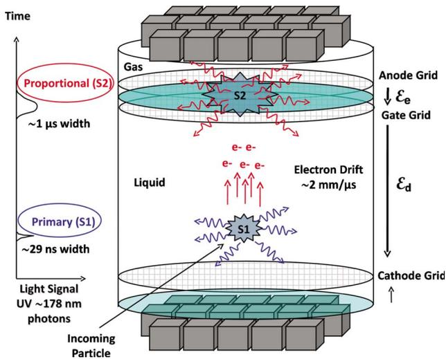
FIG. 44. (Color online) Schematic of a two-phase xenon TPC.
