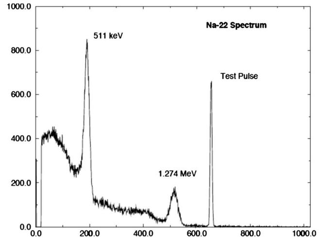
FIG. 33. The energy spectrum of  $^{22}\text{Na}$  gamma rays measured with the gridded ionization chamber shown in Fig. 30 at 4 kV/cm drift field (Aprile *et al.*, 2002). The energy resolution of the 511 keV line is about 8% (FWHM).
