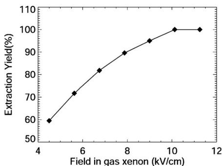
FIG. 45. Electron-extraction yield in LXe as a function of the electric field in the gas phase (Aprile *et al.*, 2004a).
