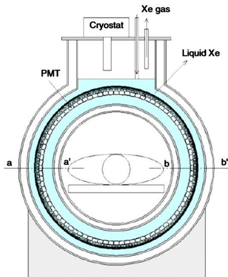
FIG. 85. (Color online) Schematic of the Waseda full scale LXe TOF-PET (Doke, Kikuchi, and Nishikido, 2006).
