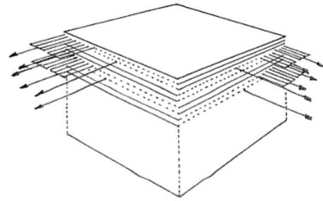
FIG. 52. Schematic of the wire electrode system for the LXe ionization calorimeter for GeV gamma rays (Doke *et al.*, 1989; Doke, Kasahara, and Suson, 1992).
