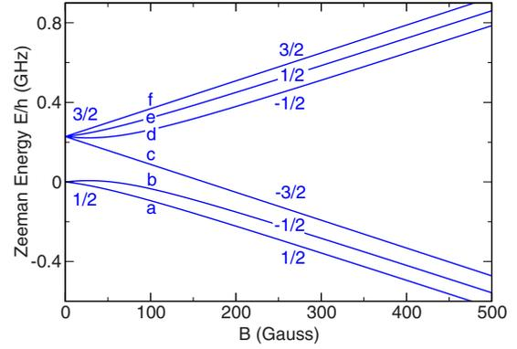
FIG. 5. (Color online) Atomic energy levels of the  $^6\text{Li}$  atom, which has  $S=1/2$ ,  $I=1$ , and  $f=1/2$  and  $3/2$ . The figure shows both the projection  $m$  of  $f$  and the alphabetical shorthand notation  $q_i=a, b, c, d, e,$  and  $f$  used to label the levels in order of increasing energy.
