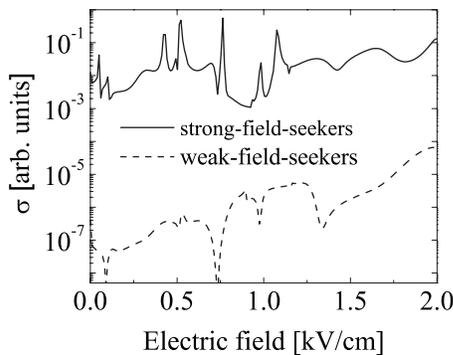
FIG. 48. Calculated chemical reaction cross section of  $\text{H}_2\text{CO} + \text{OH} \rightarrow \text{HCO} + \text{H}_2\text{O}$  at a collision energy of  $E/k_B = 1$  mK as a function of applied electric field. Strong- (weak-) field seekers correspond to states of  $\text{H}_2\text{CO}$  and OH that can be held in an electric trap where the center of the trap has the largest (smallest) electric field strength, respectively. From [Hudson \*et al.\*, 2006](#).
