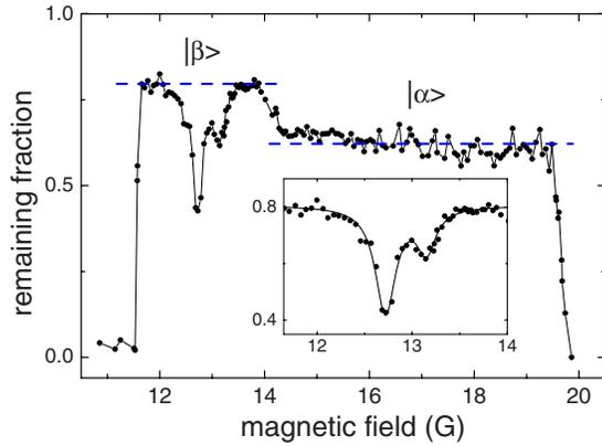
FIG. 47. (Color online) Observation of Feshbach-like resonances in the collisions of  $^{133}\text{Cs}_2$  molecules. The number of remaining  $^{133}\text{Cs}$  molecules after fixed storage time in an optical trap as a function of external magnetic field. The two features near 13 G shown magnified in the inset have been interpreted as tetramer resonances. From [Chin \*et al.\*, 2005](#).
