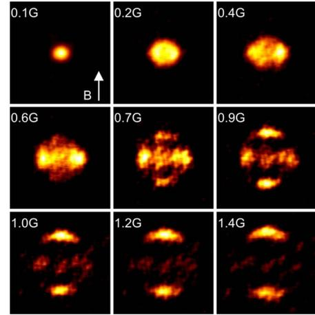
FIG. 36. (Color online) Dissociation patterns of  ${}^{87}\text{Rb}_2$  molecules, showing the interference of  $s$ - and  $d$ -partial waves. At small magnetic field offsets  $B - B_0$  (values given in the upper left corners), the  $s$ -wave pattern dominates; at large offsets,  $d$  waves are strongly enhanced due to a  $d$ -wave shape resonance. From [Volz \*et al.\*, 2005](#).
