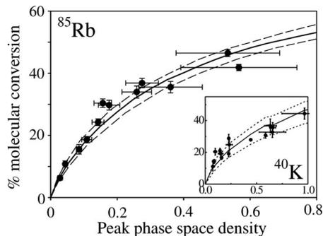
FIG. 34. Illustration of the dependence of the atom-molecule conversion efficiency on the atomic phase-space density. The main figure shows the results obtained in a near-degenerate bosonic gas of  $^{85}\text{Rb}$  atoms, while the inset shows corresponding results on a fermionic gas of  $^{40}\text{K}$  atoms. The lines refer to a theoretical model that is based on the phase-space overlap of atom pairs in the trapped gases. From [Hodby \*et al.\*, 2005](#).
