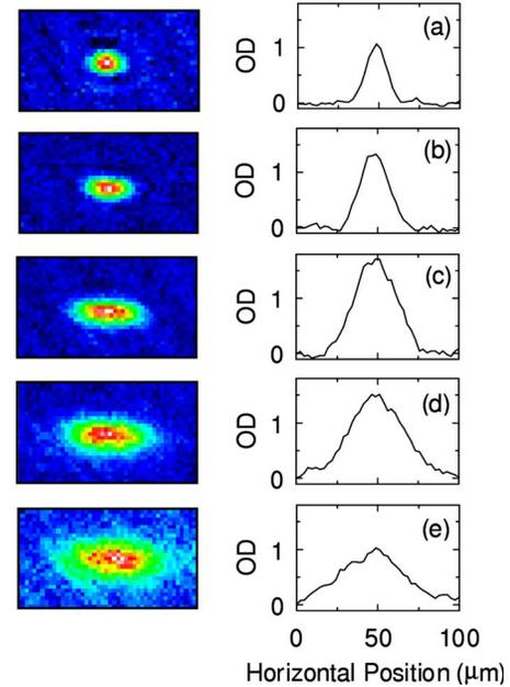
FIG. 25. (Color online) *In situ* images and density profiles showing the variation of the equilibrium size of a magnetically trapped  $^{85}\text{Rb}$  BEC close to a Feshbach resonance. With decreasing magnetic field (a)–(e), the scattering length increases from a very small positive value at 165.2 G (zero crossing at 165.8 G) to a very large value of  $a \approx +6000a_0$  at 156.4 G (resonance position at 155.0 G). From Cornish *et al.*, 2000.
