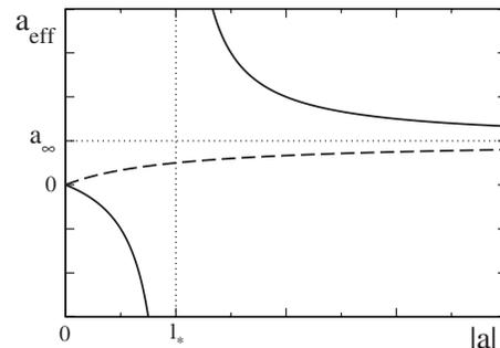
FIG. 44. The dependence of the effective scattering length  $a_{\text{eff}}$  on the absolute value of the microscopic scattering length  $|a|$ . The dashed line corresponds to a repulsive interaction potential ( $a > 0$ ). The solid line corresponds to an attractive potential ( $a < 0$ ) with a geometric resonance at  $|a| = l_*$ . From [Fedichev \*et al.\*, 2004](#).
