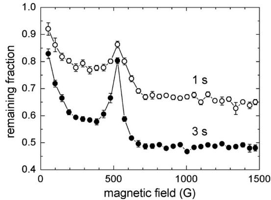
FIG. 19. Fraction of trapped atoms remaining after evaporation of  ${}^6\text{Li}$  atoms in an optical dipole trap after 1 s (open circles) and 3 s (closed circles) hold times. The peak near 530 G indicates a minimum of evaporative loss. This minimum results from the zero crossing of the scattering length induced by the broad 834 G Feshbach resonance. From [Jochim \*et al.\*, 2002](#).
