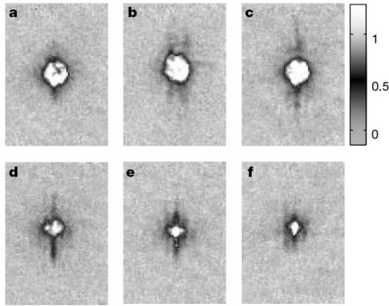
FIG. 26. Striking phenomena have been observed in the controlled collapse of a  $^{85}\text{Rb}$  BEC. The images show the formation of “jets,” where streams of atoms with highly anisotropic velocities are ejected by the collapsing condensate. From [Donley \*et al.\*, 2001](#).
