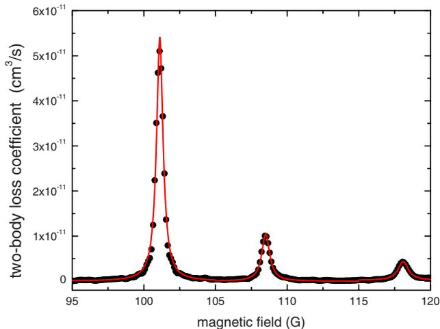
FIG. 18. (Color online) Two-body inelastic loss coefficient of cesium atoms in the  $|f=3, m=-3\rangle$  state as a function of magnetic field. The loss coefficient is extracted from the atomic density evolution, as shown in Fig 17. Three resonances are identified here. The solid line is a Lorentzian fit. From Chin, Vuletić, *et al.*, 2004.
