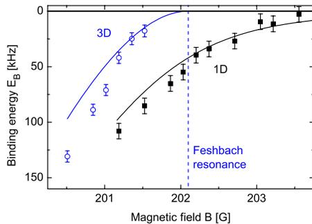
FIG. 43. (Color online) Measured molecular bound state binding energy vs magnetic field  $B$  near the 202.1 G resonance between the two lowest spin states of  $^{40}\text{K}$ . The upper curve labeled 3D is for a free space gas, whereas the lower curve labeled 1D is for a quasi-1D gas with tight confinement in two dimensions. The points show measured binding energies and the lines show theoretical predictions. From [Moritz \*et al.\*, 2005](#).
