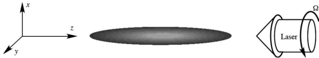
FIG. 6. A cigar-shaped condensate is confined by an axisymmetric magnetic trap and stirred by an off-center far-detuned laser beam. The laser beam propagates along the long axis and creates an anisotropic quadrupole potential that rotates at an angular velocity \Omega . From Madison et al. , 2000b .
