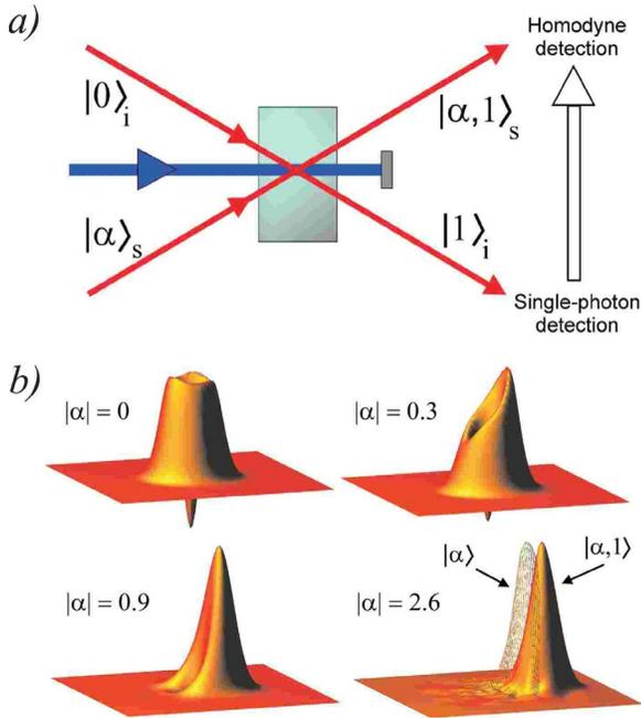
FIG. 16. (Color online) The single-photon-added coherent state. (a) Scheme of the experiment. (b) With increasing  $\alpha$ , the Wigner function of the reconstructed single-photon-added coherent state gradually evolves from a highly nonclassical to a highly classical shape. For  $|\alpha|=2.6$ , the Wigner function of the unexcited seed coherent state is also shown. From [Zavatta \*et al.\*, 2004a](#).
