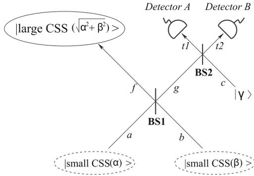
FIG. 14. A schematic for amplification of the “Schrödinger cat” state. The amplified cat emerges in channel  $g$  if detectors  $A$  and  $B$  click in coincidence. In the text,  $\alpha=\beta=\gamma/\sqrt{2}$  is assumed. From [Lund et al., 2004](#).
