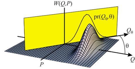
FIG. 2. (Color online) The Wigner function. The experimentally measured field quadrature probability density  $\text{pr}(Q_\theta, \theta)$  is the integral projection of the Wigner function  $W(Q, P)$  onto a vertical plane defined by the phase of the local oscillator.
