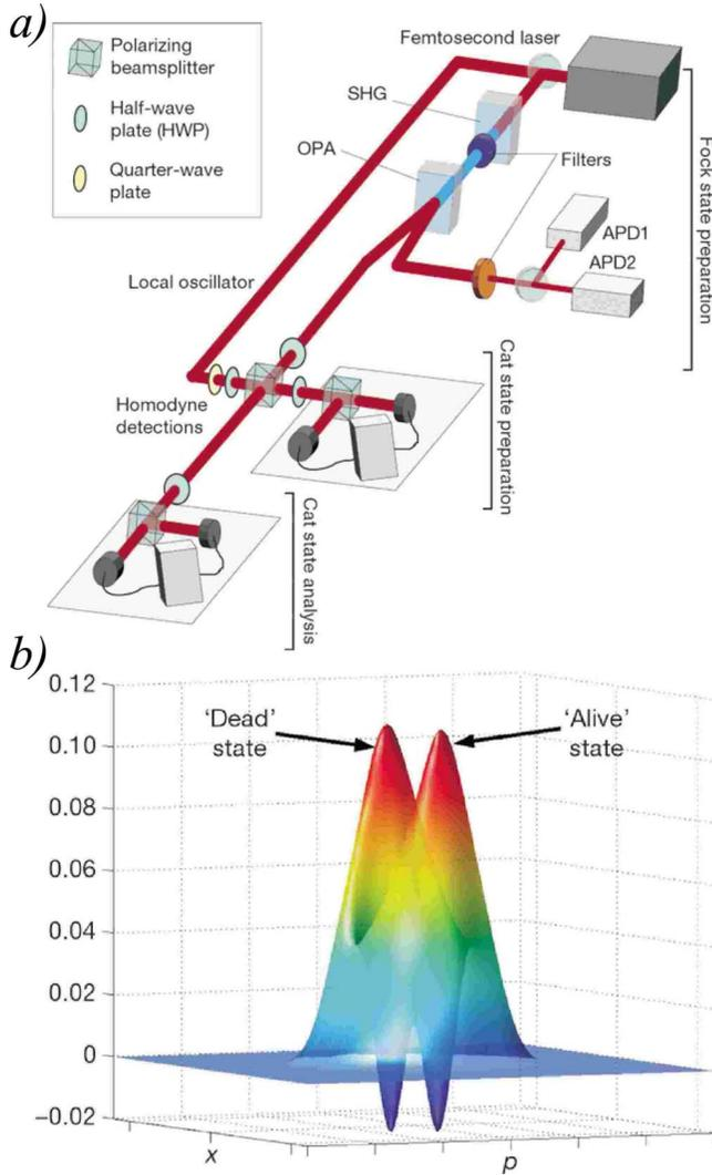
FIG. 15. (Color online) Conditional preparation of the Schrödinger cat state from photon number states. (a) A scheme of the experiment. (b) The experimental Wigner function. From [Ourjoutsev et al., 2007](#).
