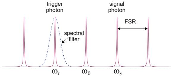
FIG. 7. (Color online) Spectrum of the Fabry-Perot parametric cavity. If one of the spectral modes ( $\omega_t$ ) is selected in the trigger channel, a click of the trigger detector heralds production of the signal photon in a pure cavity mode at  $\omega_s = 2\omega_0 - \omega_t$ .
