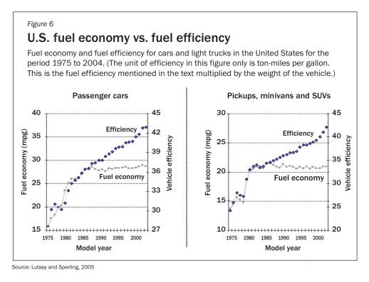
define fuel economy as vehicle miles per gallon of fuel, or how far you can go on a gallon of fuel. Where different with fuels different energy contents compared (e.g., gasoline, diesel, ethanol) the energy differences are noted. In general, economy is not equivalent to efficiency. Efficiency relates to the fraction of the energy content of fuel used to move the vehicle.
