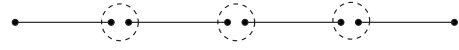
FIG. 1. Schematic of the nearest-neighbor valence bond state, exact ground state of the spin-1 model in Eq. (27) for \beta=1/3 (AKLT-model). The ground state is constructed regarding every S=1 in the lattice sites as made of a pair of S=1/2 , and projecting out the singlet state. The singlets are then formed taking pairs of S=1/2 in nearest-neighbor sites.
