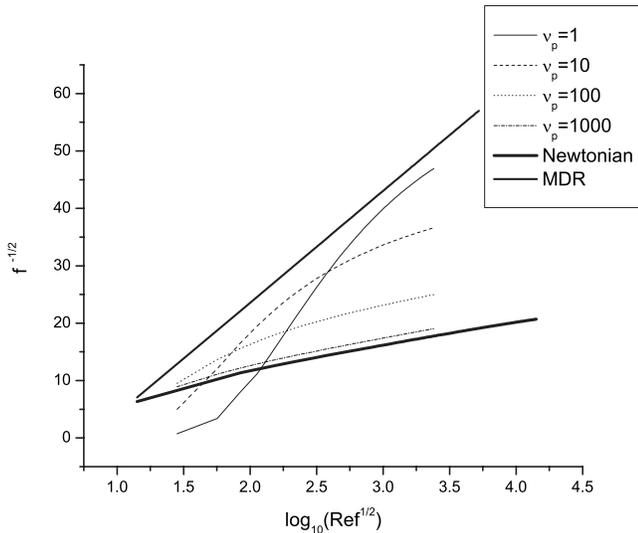
FIG. 16.  $f^{-1/2}$  as a function of  $\log_{10}(Re f^{1/2})$  with  $\lambda=1$  with various values of  $\nu_p$ .
