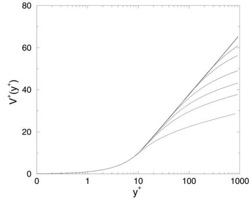
FIG. 14. The mean velocity profiles for flexible polymer additives with  $\tilde{\nu}=1, 5, 10, 20, 50, 100$ , and  $500$  from below to above. Note that the profile follows the MDR until it crosses over back to the Newtonian plug.
