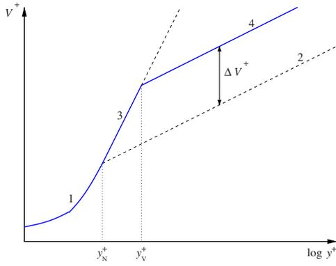
FIG. 12. (Color online) Schematic mean velocity profiles. Region 1,  $y^+ < y_N^+$ , viscous sublayer. Region 2,  $y^+ > y_N^+$ , logarithmic layer for the turbulent Newtonian flow. Region 3,  $y_N^+ < y^+ < y_V^+ = (1+Q)y_N^+$ , MDR asymptotic profile in the viscoelastic flow. Region 4,  $y^+ > y_V^+$ , Newtonian plug in the viscoelastic flow.
