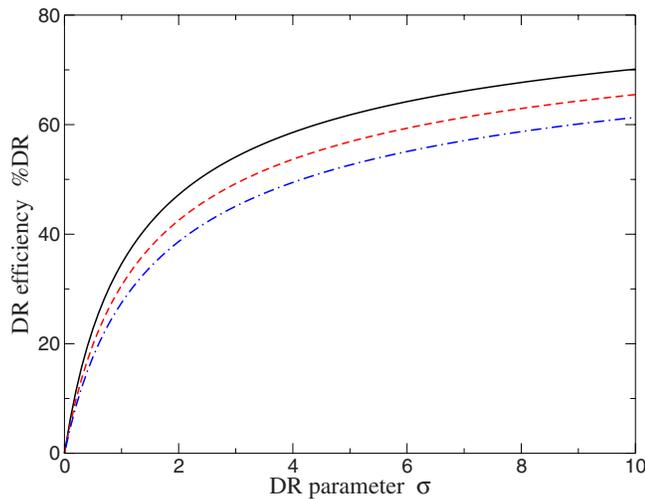
FIG. 13. (Color online) Drag reduction efficiency %DR as function of the drag reducing parameter  $Q$  for different centerline Reynolds numbers  $Re$ :  $1.2 \times 10^5$ ,  $1.2 \times 10^6$ , and  $1.2 \times 10^7$  (from top to bottom).
