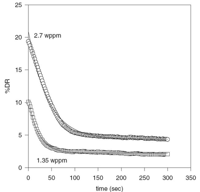
FIG. 3. %DR in a counter-rotating disks experiment with  $\lambda$ -DNA as the drag reducing polymer. Note that the %DR is proportional to  $c_p$ . When the length  $N_p$  reduces by a factor of 2 and, simultaneously,  $c_p$  increases by factor of 2, the %DR reduces by a factor of 4.
