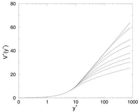
FIG. 15. The mean velocity profile for rodlike polymer additives with  $\tilde{\nu}=1, 5, 10, 20, 50, 100, 500, 1000, 5000,$  and  $10\,000$  from below to above. Note the typical behavior expected for rodlike polymers, i.e., the profile diverges from the von Kármán log law, reaching the MDR only asymptotically.
