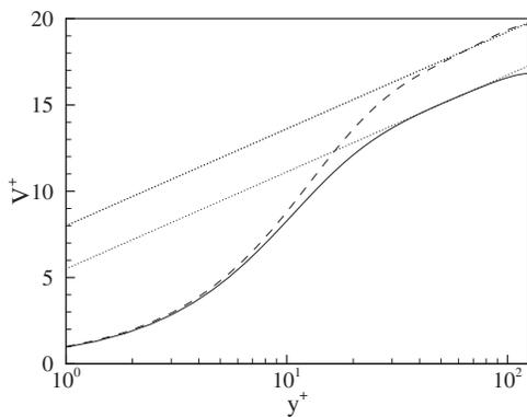
FIG. 7. Mean velocity profiles for the Newtonian and for the viscoelastic simulations with  $Re=125$  (Benzi *et al.*, 2006). Solid line, Newtonian. Dashed line, viscoelastic. Straight lines represent a log law with the classical von Kármán slope. Notice that in this simulation the modest Reynolds number results in an elastic layer in the region  $y^+ \leq 20$ .
