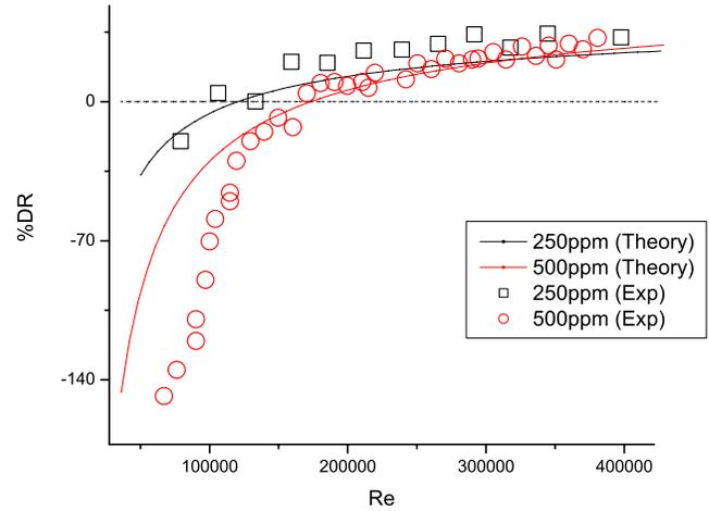
FIG. 17. (Color online) Percentage drag reduction as a function of  $Re$  for two values of the concentration of the rodlike polymer. Symbols are results of experiments and solid lines are theory, cf. [Amarouchene et al. \(2007\)](#).
