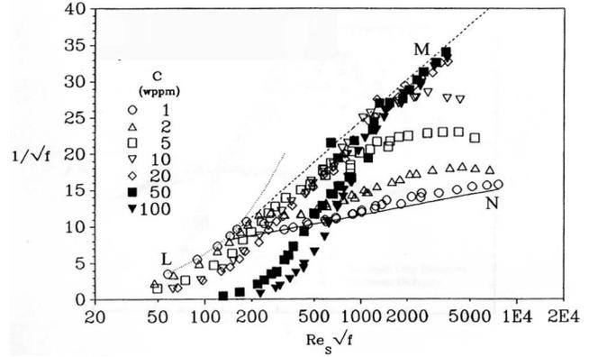
FIG. 5. The drag in Prandtl-Kármán coordinates for a low concentration solution of NaCl in water mixed with the rodlike polymer PAMH B1120 in a pipe flow, see Virk *et al.* (1996) for details. The symbols represent the concentrations in wppm (weight parts per million) as given.
