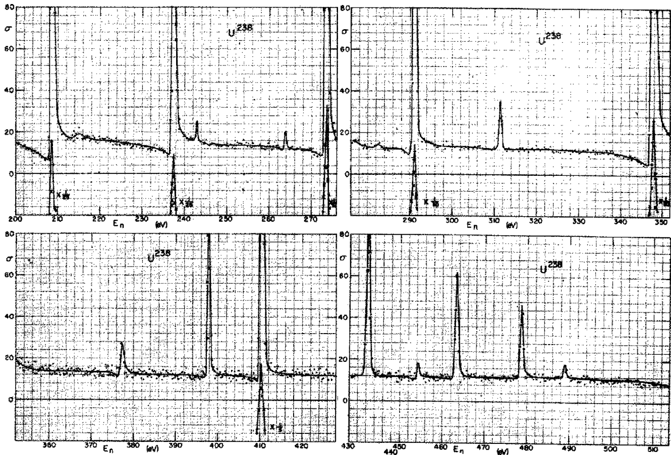
FIG. 3. Total cross section for scattering of neutrons by ^{238}\text{U} vs neutron energy. The abscissa spans about 80 eV in each of the four plots. From Garg et al. , 1964.
