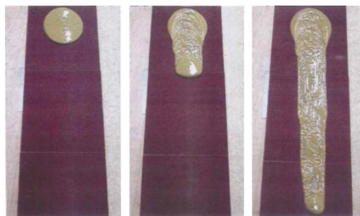
FIG. 56. (Color online) Sequence of snapshots illustrating the evolution of a clay suspension drop poured over sandpaper. From Coussot, Nguyen, et al. , 2002.
