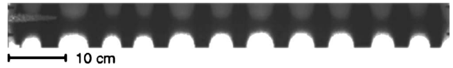
FIG. 38. Image of a shish-kebab-like structure of smaller particles in a rotating drum (illuminated from below). Smaller particles (shown in dark) form bands between bands of larger particles (disconnected rings, shown in white and gray). From Arndt et al. , 2005.
