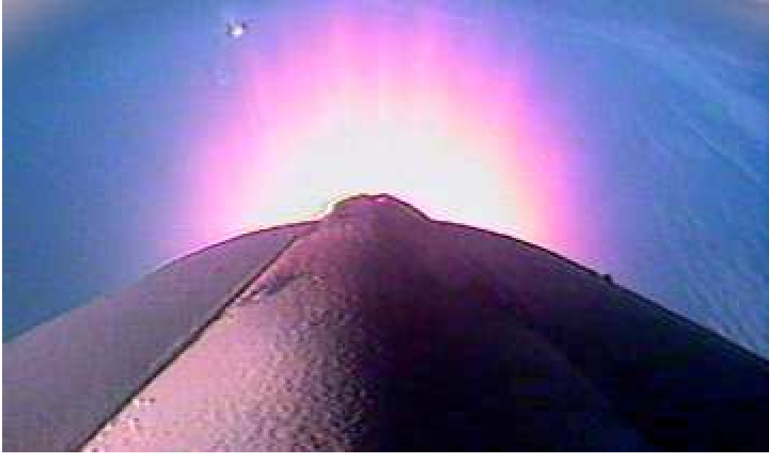
Figure 10.15. The plume from a solid-propellant Pegasus rocket, just after first-stage separation. The plume might be sufficiently opaque to have some effect on LIDAR interrogation. Courtesy of Orbital Sciences Corporation.
