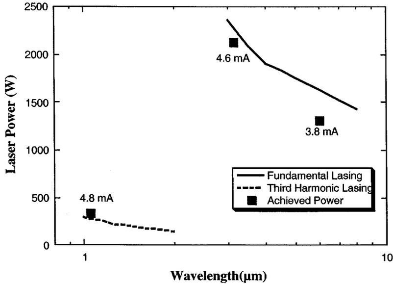
FIG. 10. Projected and achieved performance of the IR demonstration FEL at Jefferson Laboratory. The full available performance can be achieved by using specialized mirrors for each wavelength band. Calculations by S. Benson.
