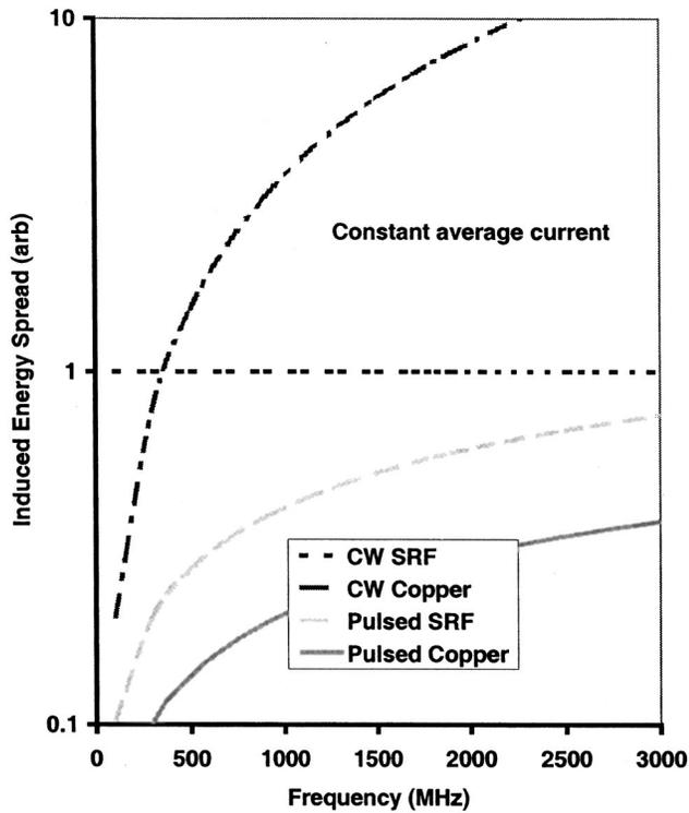
FIG. 4. Total longitudinal heating in arbitrary units as a function of frequency. The scaling has assumed a fixed total energy  $\langle I \rangle$ ,  $R/Q$ 's for each system are the values quoted in the text, and micropulse length and cavity geometry  $\sim 1/f$ . This illustrates the frequency dependence in Eq. (5).
