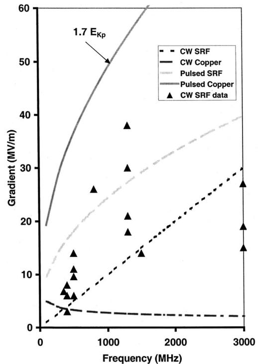
FIG. 3. Gradient limits for pulsed and continuous-wave copper and superconductive rf (SRF) linacs assumed in the stability calculations below with some illustrative recent SRF results.  $E_{Kp}$  is the Kilpatrick limit specified in Eq. (6).
