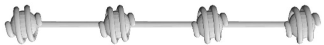
FIG. 4. Self-assembled complex of a negative polyelectrolyte molecule and many positive spheres in a necklacelike structure. On the surface of a sphere, neighboring polyelectrolyte turns are correlated similar to the rods in Fig. 8 below. On a larger scale, charged spheres repel each other and form a one-dimensional Wigner crystal along the polyelectrolyte molecule.
