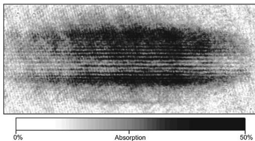
FIG. 15. Interference pattern of two expanding condensates observed after 40 ms time of flight. The width of the absorption image is 1.1 mm. The interference fringes have a spacing of  $15 \mu\text{m}$  and are strong evidence for the long-range coherence of Bose-Einstein condensates.
