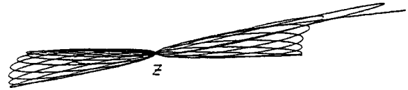
FIG. 4. Typical classical out-of-phase motion of the electron pair in helium obtained from a numerical integration of the full Hamilton equations of motion. The electrons evolve on perturbed Kepler ellipses around the nucleus until they autoionize after a few revolutions (from Richter, 1991).
