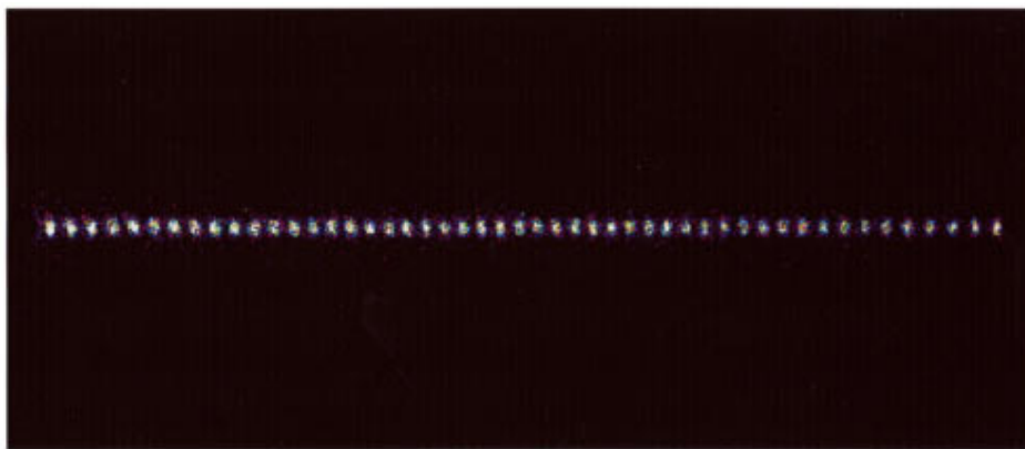
FIG. 5. (Color) Linear chain of ions in a trap. The position of the ions is marked through the fluorescence radiation. They are constantly emitting when illuminated by a laser beam. The laser beam is used simultaneously to cool the ions so that they stay in an ordered configuration. Such an ion chain has been proposed as the register of a quantum computer.
