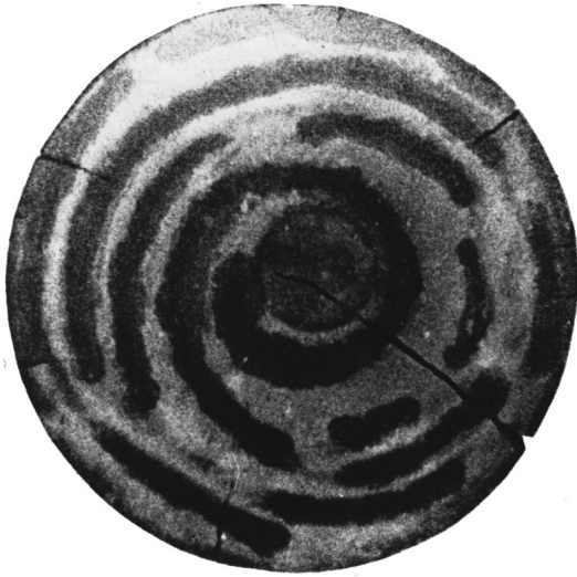
FIG. 20. Photograph of the burnt disk. The front traveled from the center to the periphery. Traces of the reaction spot appear on the surface. From Merzhanov et al. (1982).
