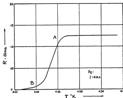
FIG. 2. Onnes' curve for mercury.
