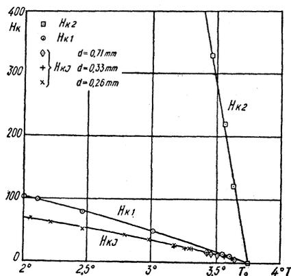
FIG. 22. Critical magnetic fields for  $\text{PbTl}_2$ .
