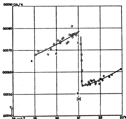
FIG. 16. Undisturbed (no external field) specific heat of tin.
