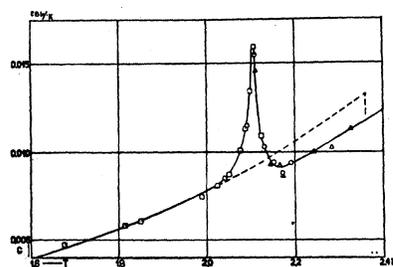
FIG. 17. Specific heat of thallium in a magnetic field.
