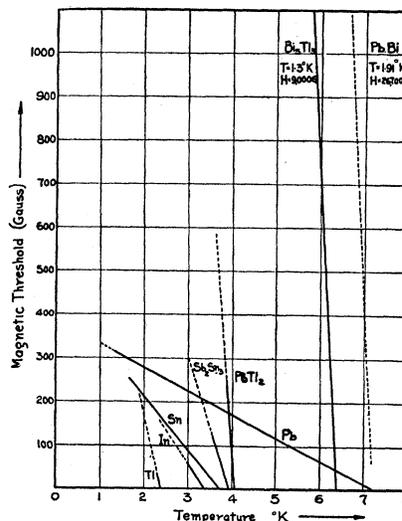
FIG. 6. Magnetic threshold fields for superconductors.
