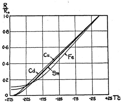
FIG. 1. Change of resistance with temperature.
