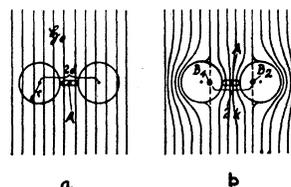
FIG. 9. Parallel cylinders. (a) Normal. (b) Superconducting.
