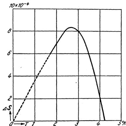
FIG. 24. Entropy difference between normal and superconducting states for mercury.
