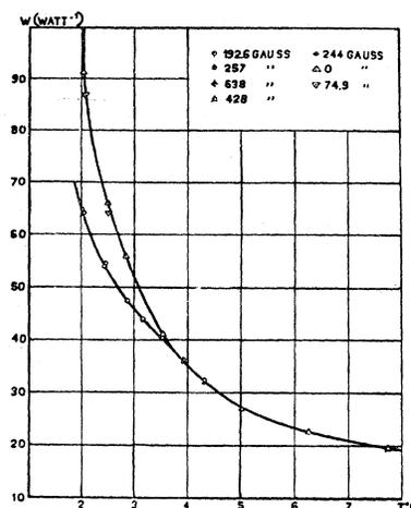
FIG. 18. Thermal resistance with and without magnetic field.
