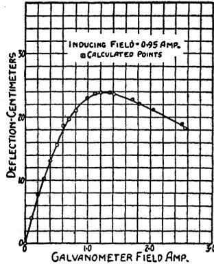
FIG. 15. Experimental test of superconducting galvanometer.
