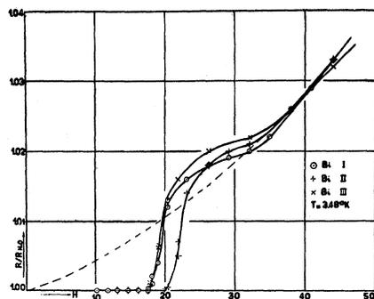
FIG. 11. Penetration of a magnetic field into a tin cylinder.
