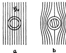
FIG. 8. Hollow cylinder. (a) Normal. (b) Superconducting.
