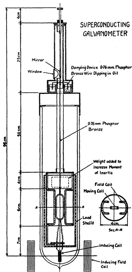
FIG. 14. Superconducting galvanometer.
