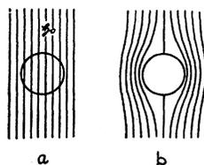
FIG. 7. Cylinder in a magnetic field. (a) Normal. (b) Superconducting.
