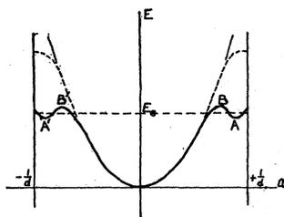
FIG. 25. Suggested energy-momentum curve for a superconductor (dotted curve—"nearly free" electrons).
