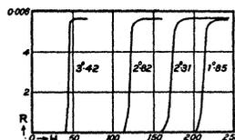
FIG. 3. Dependence of resistance on magnetic field.
