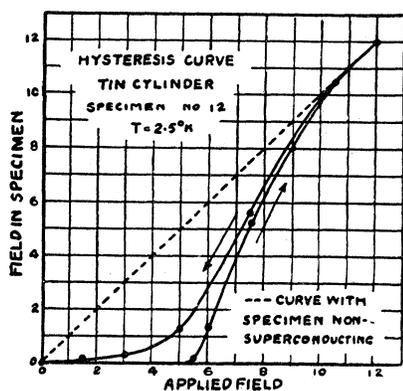
FIG. 12. Magnetic hysteresis curve for a tin cylinder.
