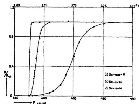
FIG. 4. Transition curves for monocrystalline and polycrystalline tin.
