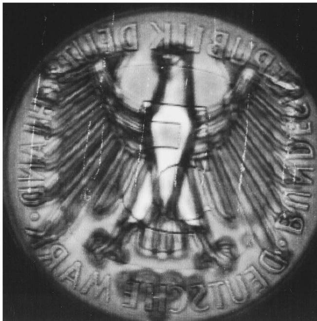
FIG. 4. An acoustic image of a 5-DM German coin at 10 MHz (Leica, Wetzlar).
