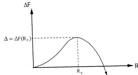
FIG. 3. Schematic of the total energy of a bubble of  $B$  phase in supercooled  $A$  phase as a function of the radius of the bubble. The energy increases with increasing bubble size for  $R < R_c$ , due to the surface tension, and then decreases for  $R > R_c$ .
