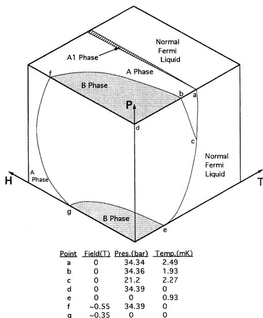
FIG. 1. Schematic of the equilibrium phase diagram of superfluid  $^3\text{He}$  (proportions are not scaled accurately). The top plane is the solid-liquid phase boundary. The  $B$  phase is preferred at lower temperatures than the  $A$  phase, but completely excluded at high magnetic fields (Greywall, 1986; Hahn, 1993).
