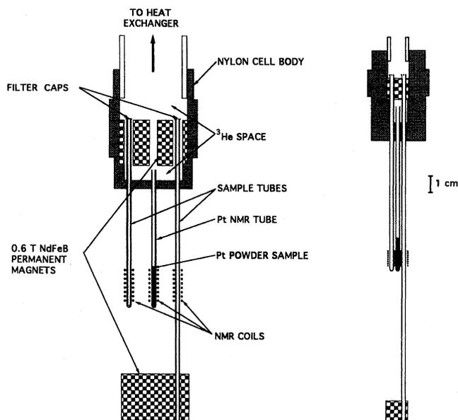
FIG. 5. Sample cell used in the  $AB$  nucleation experiments. The drawing on the left has been distorted for labeling purposes, while the drawing on the right shows the correct aspect ratio. Two empty tubes were used to study the transition, while a third contained Pt powder for Curie-law thermometry.
