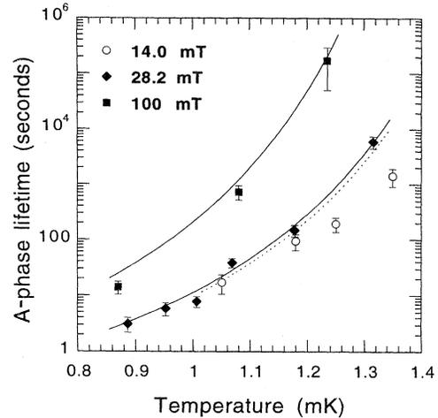
FIG. 8. Temperature dependence of the lifetime of the metastable  $A$  phase in the presence of the  $^{60}\text{Co}$  source at three different magnetic fields. The fits are described in the text. The function does not fit the high-temperature data at 14 mT well, suggesting that a parallel nucleation mechanism may be active.
