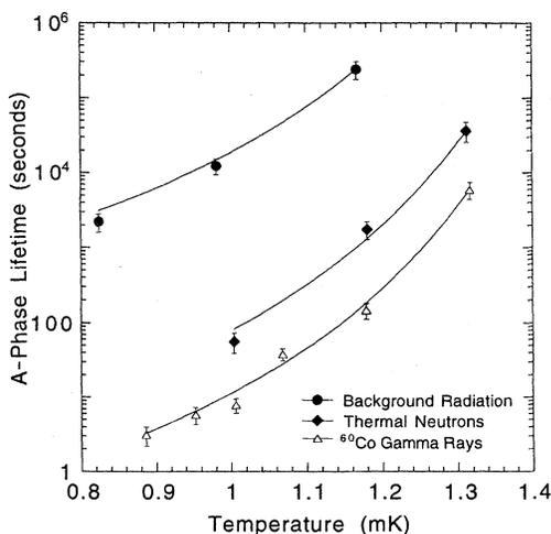
FIG. 7. Lifetime of the metastable  $A$  phase as a function of temperature in a magnetic field of 28.2 mT with different ionizing radiations incident on the samples. All three data sets are fit to the same functional form as discussed in the text and shown by the solid lines. These were obtained by fitting the functional form to the gamma-ray data and then multiplying by constant factors of 7 and 1650 to fit the neutron and background data, respectively.
