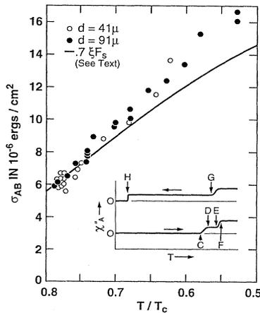
FIG. 2. Surface energy at the  $AB$  interface as a function of temperature; the inset shows raw data taken in the experiment (Osheroff and Cross, 1977).
