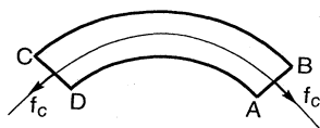
FIG. 16. Control volume ABCD (bold curves) around an interface (thin curve). The capillary forces f_c act on the control volume.
