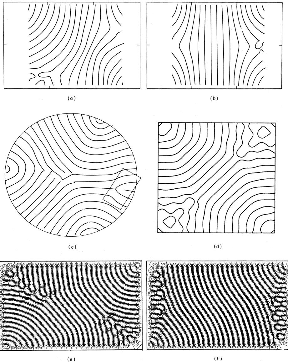
FIG. 3. Horizontal spatial patterns in convection with lateral boundaries; (a) and (b) are from experiments of Gollub *et al.* (1982); (c) from experiments of Croquette *et al.* (1983); and (d)–(f) from numerical simulations of the Swift-Hohenberg model equation (3.27) by Greenside and Coughran (1984).
