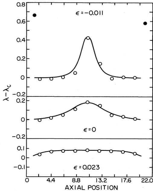
FIG. 62. Local wavelength (vortex-pair width) of Taylor vortices in a system of aspect ratio  $L = 21.27$  containing 10 vortex pairs, as a function of axial position, for three values of the reduced control parameter  $\epsilon$ . The solid circles in the top panel represent the Ekman vortex adjacent to each boundary. The solid lines follow from Eq. (9.37). (From Ahlers *et al.*, 1986.)
