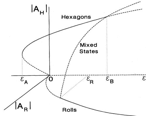
FIG. 10. Amplitude of roll state  $|A_R|$  and hexagon state  $|A_H|$  as function of control parameter  $\varepsilon$ , following from Eq. (4.40). Solid lines denote stable states, dashed lines unstable states. The limits of stability  $\varepsilon_A, \varepsilon_B$ , and  $\varepsilon_R$  are given in Eq. (4.41). (From Ciliberto *et al.*, 1990.)
