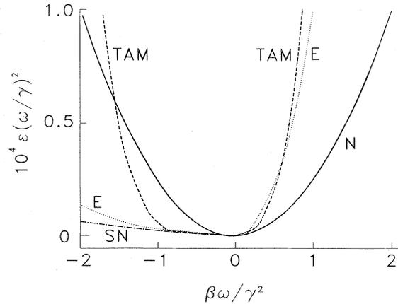
FIG. 70. Stability boundaries for square patterns of standing surface waves as a function of the control parameter  $\epsilon$  and the detuning parameter  $\beta$  which is a representation of the wave vector  $q$  [see Eq. (9.95)]. Solid line (N), neutral stability boundary; dotted line (E), Eckhaus boundary; dashed line (TAM), transverse amplitude modulation; dash-dotted line (SN), saddle-node point for subcritical bifurcation. (From Milner, 1991.)
