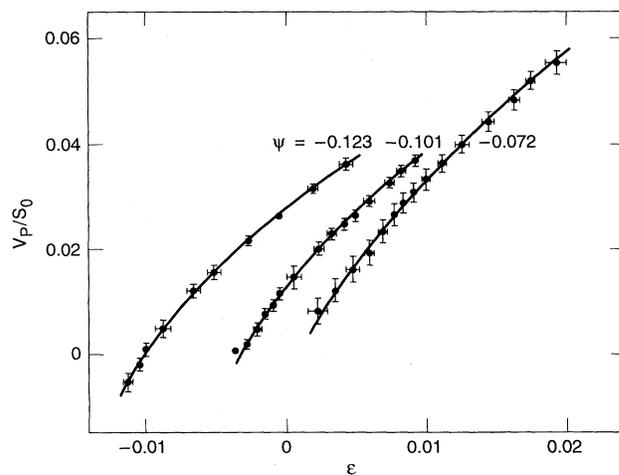
FIG. 57. Pulse velocity  $v_p$  normalized by the linear group velocity  $s_0$  vs control parameter  $\epsilon$ , for pulses such as the one in Fig. 56 and different binary-fluid mixtures. The reduced velocity is seen to be very small in magnitude and to depend on the fluid parameters. (Adapted from Kolodner, 1991d.)
