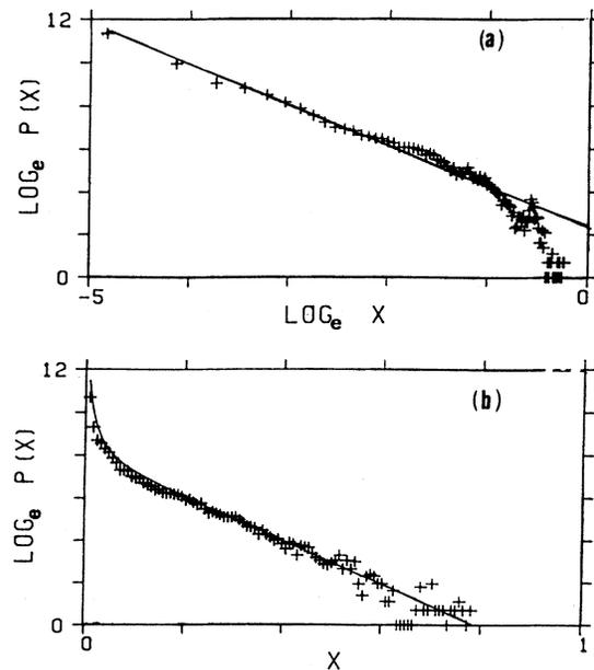
FIG. 46. Distribution  $P(x)$  of “laminar” domains of length  $x$  for convection in a long thin annulus. (a) At reduced control parameter  $\varepsilon = 240$  the line shows algebraic decay with exponent 1.9. (b) As in (a) but for  $\varepsilon = 309$ , now showing an exponential decay with decay length  $\xi \approx 0.1$ . (From Ciliberto and Bigazzi, 1988.)
