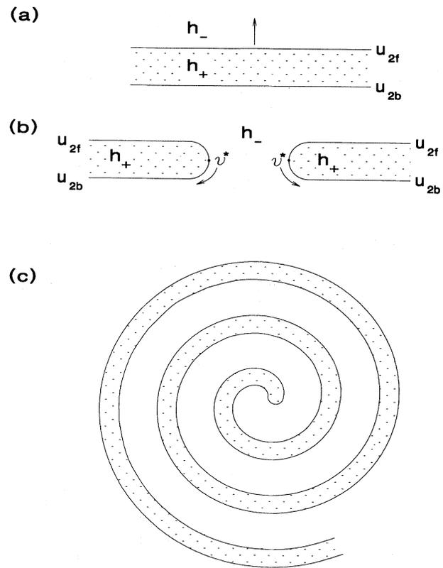
FIG. 82. Schematic illustration of spiral pattern dynamics. (a) and (b) Formation of a spiral by breaking a propagating pulse. Regions of high  $u_1$  concentration are shown hatched. (c) Completed single spiral. See text for details.
