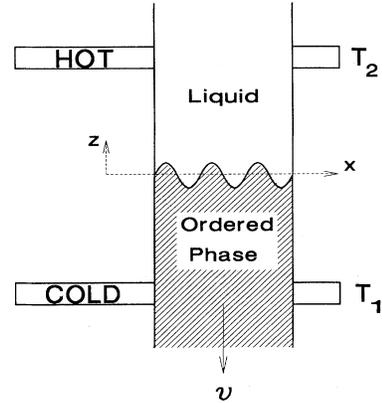
FIG. 102. Directional solidification geometry. Two microscope slides containing a thin film of the material are drawn at a constant velocity  $v$  between a hot oven at temperature  $T_2$  and a colder oven at temperature  $T_1$ , bracketing the transition temperature between ordered and disordered phases.
