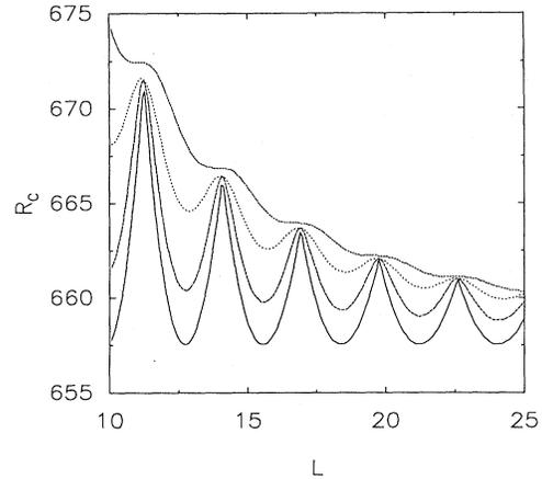
FIG. 13. Threshold Rayleigh number  $R_c$  for onset of convection in a one-dimensional system of size  $L$  for the model of free-slip convection. The boundary conditions at the ends interpolate from free-slip thermal insulators (bottom line) to rigid good thermal conductors (top line). (From Y.-Y. Chen, 1992.)
