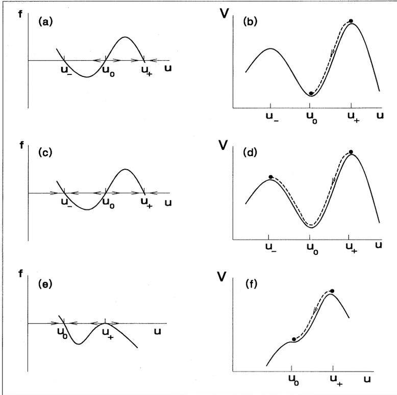
FIG. 17. Illustration of various forms of  $f(u)$  and the associated  $V(u)$  for the nonlinear diffusion equation (5.64). Arrows in (a), (c), and (e) show stability of fixed points  $u_+, u_0, u_-$  corresponding to spatially independent solutions. Trajectories in (b), (d), and (f) (dashed lines) correspond to coherent structures of the *pde* (5.63).
