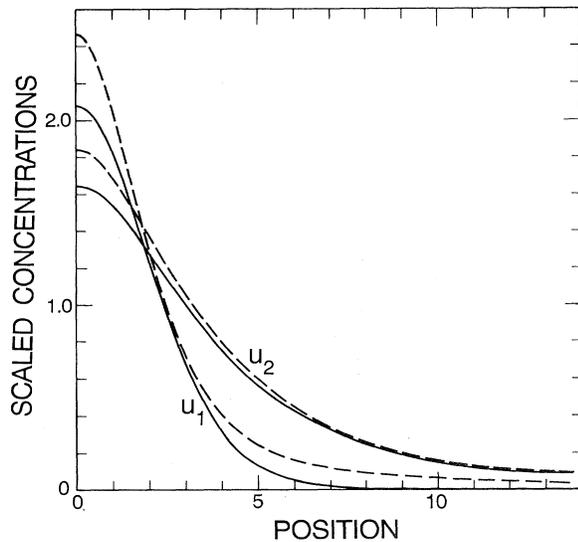
FIG. 91. Solutions for scaled activator concentration  $u_1$  and inhibitor  $u_2$  as a function of position, in the presence of inhomogeneous source terms used by Gierer and Meinhardt (1972), Eq. (11.7) (full lines). The dashed lines show the relaxation if the source terms are subsequently eliminated [i.e.,  $s(x) \rightarrow 0$ ,  $\rho(x) \rightarrow 1$ ].
