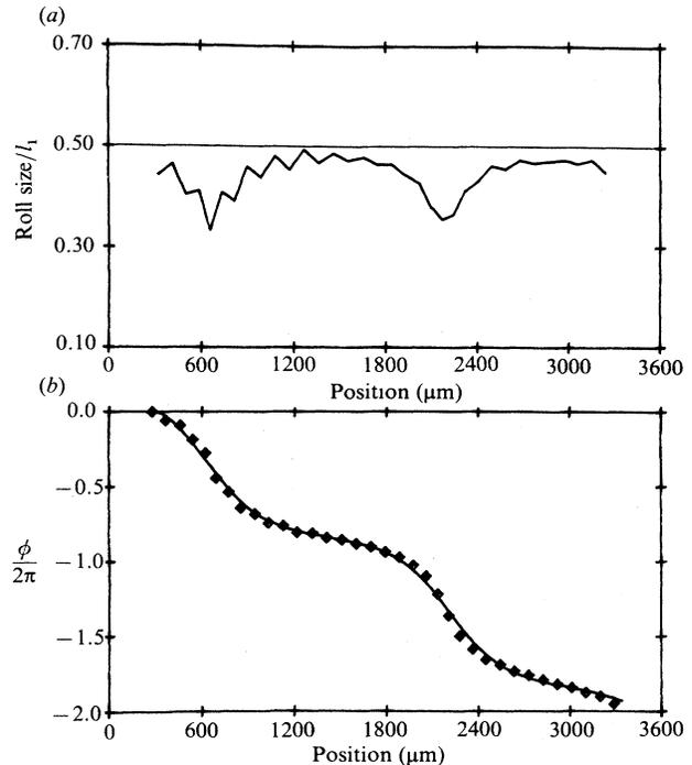
FIG. 66. Spatially forced electrohydrodynamic convection. (a) Roll size (in units of the wavelength  $\ell_1$  of the forcing) as a function of the position across the cell. Note that over large regions the pattern is nearly commensurate at  $\ell = \ell_1/2$ , with compressed regions in between. (b) Variation of the phase of the complex amplitude across the sample. The solid line is a fit to Eq. (9.54). (From Lowe *et al.*, 1986.)
