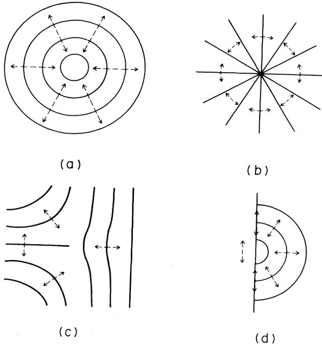
FIG. 20. Schematic diagram of disclination point defects: (a) Focus singularity (strength +1). (b) Alternate +1 defect. (c) Defect of strength  $-1/2$ . (d) Disclination on lateral sidewall. The full lines denote phase contours (rolls), the dashed arrows are the normals to the rolls.
