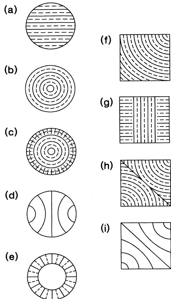
FIG. 21. Schematic of possible patterns in Rayleigh-Bénard convection and other type  $I_s$  systems. Solid and dashed lines represent roll boundaries (e.g. upflow and downflow, respectively). In (d) and (i) only a coarse grained representation of the roll boundary directions is shown, and there are many dislocations on a finer scale not shown, which permit the large scale distortions.
