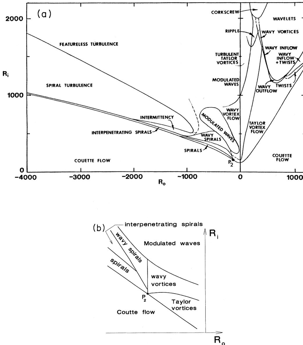
FIG. 58. Diversity of flow regimes observed in the Taylor-Couette system with independently rotating cylinders. (a)  $R_i$  and  $R_o$  are the Reynolds numbers, proportional to the rotation rates, of the inner and outer cylinders, respectively (from Andereck *et al.*, 1984). (b) Schematic expansion of the region around the codimension-two point  $P_2$  at  $R_i = -100$ ,  $R_o = 200$ , analyzed by Chossat and Iooss (1985).
