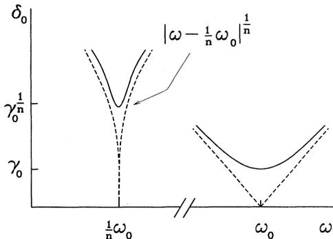
FIG. 68. Neutral stability curves in the driving strength  $\delta_0$  vs frequency  $\omega$  plane for the Mathieu equation (9.65) with parameters defined in (9.68) (only the first and the  $n$ th tongues are shown). Instability occurs above the full curves for nonzero damping  $\gamma_0$ . For  $\gamma_0 = 0$  the instabilities occur above the dashed lines.
