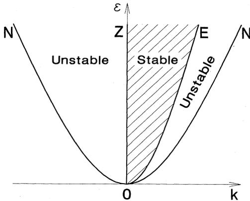
FIG. 9. Stability boundaries from amplitude equation (4.13), showing reduced control parameter vs deviation of wave vector from its critical value,  $k = q - q_0$ . N neutral; E Eckhaus; Z zig-zag. Hatched region is stable to small perturbations.
