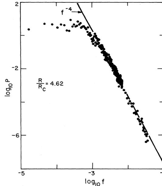
FIG. 44. Power spectral density of temperature fluctuations  $\Delta T/\Delta T_c$  in  $\text{Hz}^{-1}$  across a small aspect ratio cylindrical convection cell ( $L=4.72$ ) maintained at constant heat flux, as a function of frequency in  $\text{Hz}^{-1}$  on a log-log plot. The Rayleigh number and Prandtl number are  $R/R_c=4.62$  and  $\sigma=0.7$ , respectively. Note the power-law falloff at high frequencies. (From Ahlers and Behringer, 1978.)
