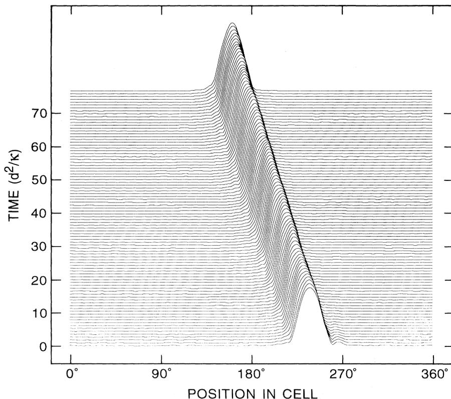
FIG. 56. Drifting pulse in annular convection cell of dimensionless circumference  $L=92$ , containing an alcohol-water binary mixture with separation ratio  $\psi=-0.12$ . Space-time plot of the envelope of the shadowgraph signal representing a localized pulse of convection embedded in a conducting background. The pulse drifts slowly to the left. (From Kolodner, unpublished).
