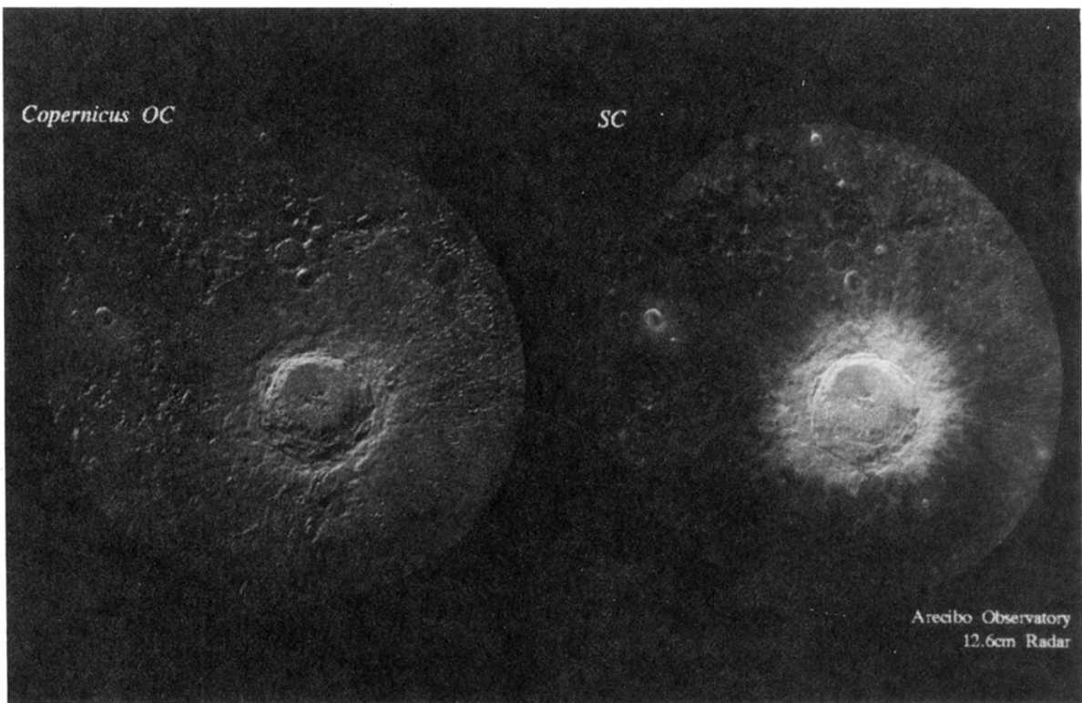
FIG. 16. Arecibo OC and SC delay-Doppler maps of the 93-km-diameter lunar crater Copernicus ( 10^{\circ} N, 20^{\circ} W), courtesy of N. J. S. Stacy and D. B. Campbell. The resolution is 900 m.
