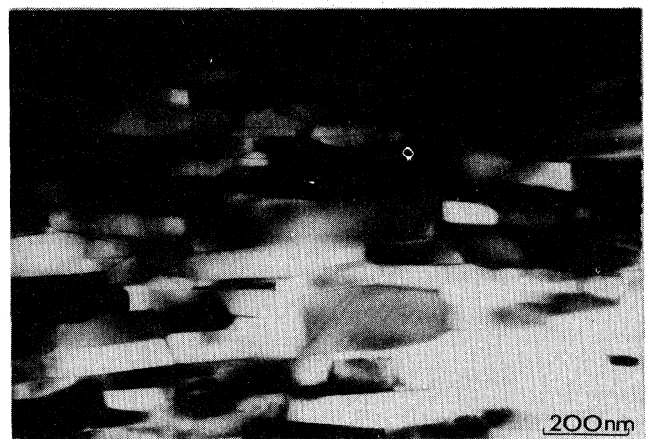
FIG. 24. Transmission electron micrograph of a die-upset Nd-Fe-B magnet (courtesy R. K. Mishra).
