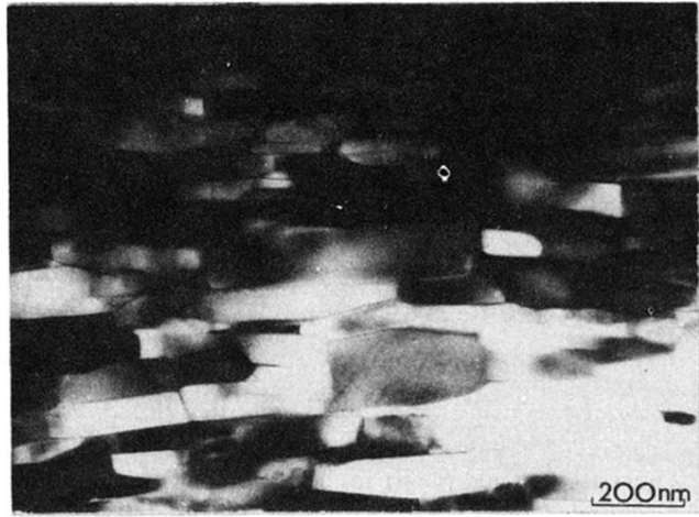
FIG. 24. Transmission electron micrograph of a die-upset Nd-Fe-B magnet (courtesy R. K. Mishra).
