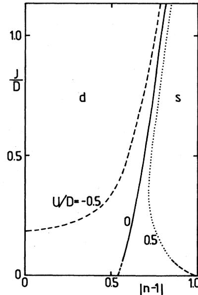
FIG. 20. Relative stability of  $s$ - and  $d$ -wave pairings for a square lattice in a plot of  $J/D$  vs  $|n-1|$ , where  $J$  measures the nearest-neighbor antiferromagnetic exchange interaction ( $W = 0$ ): solid curve,  $U = 0$ ; dashed curve,  $U/D = -0.5$ ; dotted curve,  $U/D = 0.5$ . The solid and dotted lines are extrapolated down to  $J/D = 0$ , which is shown by the dashed parts.
