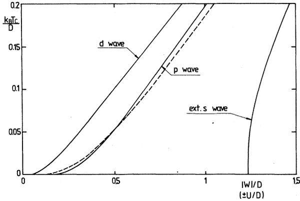
FIG. 14.  $T_c$  for  $d$ -,  $p$ -, and extended  $s$ -wave pairings on a square lattice with  $n=1$  (nearest-neighbor hopping). The dashed curve indicates  $T_c$  for both on-site ( $s$ ) pairing vs  $-U/D$  and spin-density waves vs  $U/D$  (repulsion-attraction symmetry).
