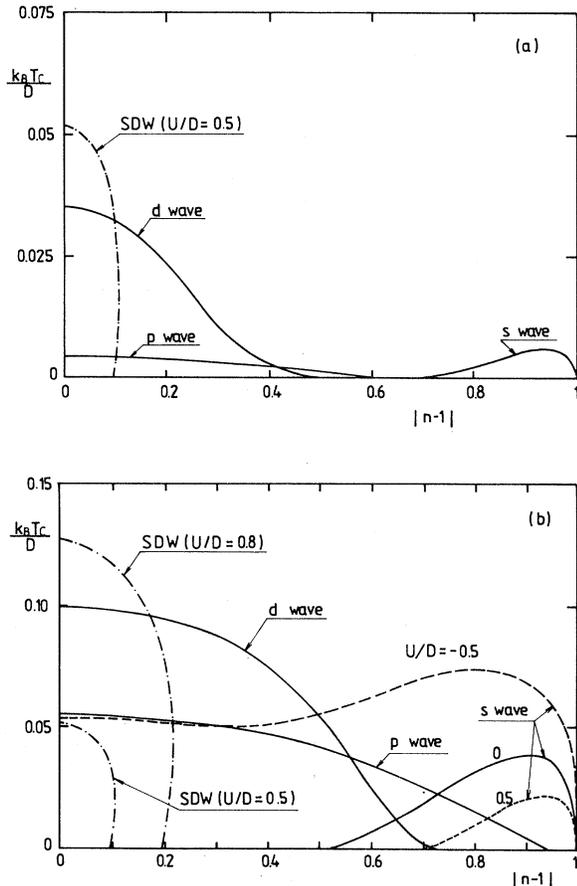
FIG. 16.  $T_c$  vs  $n$  for  $s$ -,  $p$ -, and  $d$ -wave pairings on a square lattice and with nearest-neighbor hopping.  $T_c$  for  $s$ -wave pairing is plotted for different values of  $U/D$ . Notice that  $T_c$  for  $p$ - and  $d$ -wave pairings is independent of  $U$ . (a)  $|W|/D=0.25$  ( $T_c^s$  is for  $U=0$ ), (b)  $|W|/D=0.5$ . The dot-dashed curves mark  $T_N$  for the spin-density wave state.
