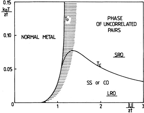
FIG. 3. Phase diagram of the half-filled Hubbard model with intra-atomic attraction ( $|U| \gg W$ ), for a simple cubic lattice (after Robaszkiewicz *et al.*, 1981a).  $T_c$  and  $T_p$  denote the critical temperatures for the onset of long-range ordering and for the breaking of electronic pairs, respectively. SRO is short-range ordering in the region of uncorrelated pairs, which is semiconducting and diamagnetic.  $2zt$  is the bandwidth.
