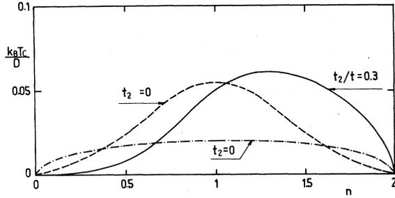
FIG. 19. Effects of next-nearest-neighbor hopping on  $T_c$  for the  $U < 0$  Hubbard model on a square lattice,  $U/D = -0.5$ ,  $D = 4t$ ; solid curve,  $t_2/t = 0.3$ ; dashed curve,  $t_2 = 0$ ; dot-dashed curve,  $T_c$  vs  $n$  for a square density of states and nearest-neighbor hopping.
