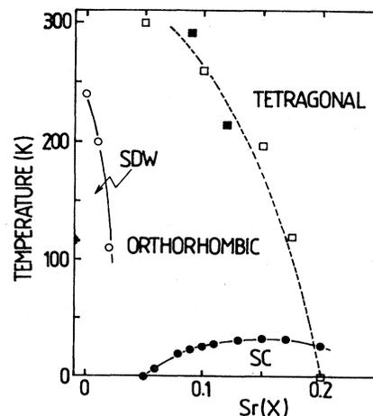
FIG. 31. Phase diagram of  $\text{La}_{2-x}\text{Sr}_x\text{CuO}_{4-\delta}$ : ●, the superconducting transition; ○, the SDW transition; ■ and □, the orthorhombic-tetragonal phase transition. The dashed lines are guides for the eye. The superconductivity at  $x \leq 0$  is not indicated on this diagram, as it concerns only a small fraction of the sample volume in which the carrier concentration does not correspond to "pure"  $\text{La}_2\text{CuO}_4$  (after Jérôme *et al.*, 1988).
