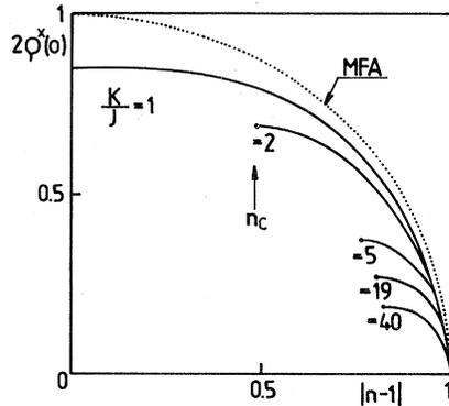
FIG. 7. Concentration dependence of the order parameter at  $T=0$  K for a local pair superconductor, for different values of  $K/J$  determined within the random-phase approximation. For  $n > n_c$  the M phase exists.
