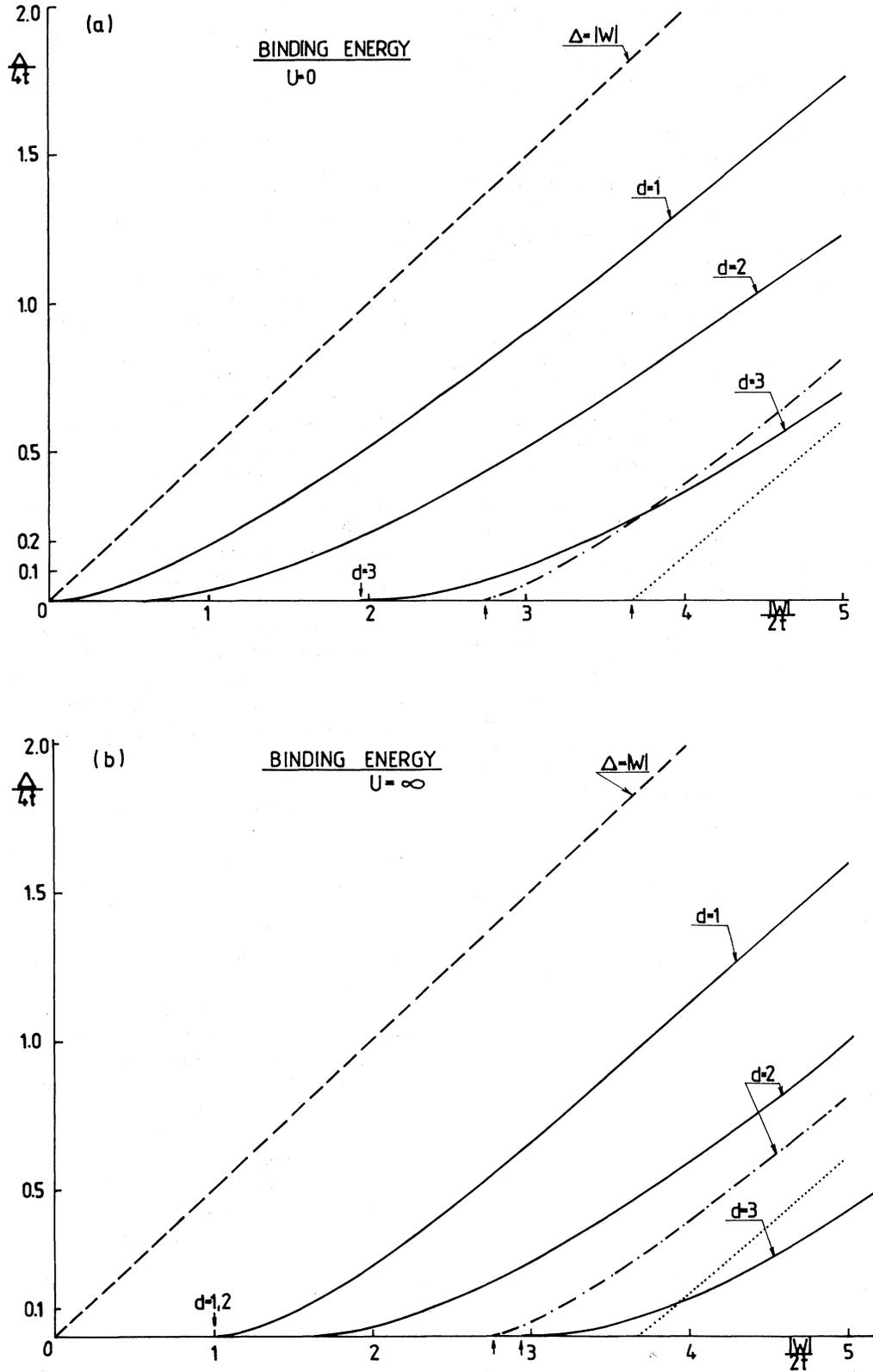
FIG. 24. Binding energies of intersite local pairs vs  $|W|/2t$  for dimensionalities  $d=1, 2, 3$ ; solid curves, s-wave pairs; dotted curve,  $d$ -wave pairs for  $d=2$ ; dot-dashed curve,  $p$ -wave pairs for  $d=2$ . A square lattice is assumed for the 2D results and a simple cubic lattice for the 3D results. (a)  $U=0$ , (b)  $U=\infty$ .
