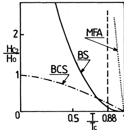
FIG. 10. Temperature dependence of the upper critical field  $H_{c_2}$  for a local pair superconductor: dotted curve, the MFA result of Bulaevskii *et al.* (1984); solid curve (BS), upper critical field for a charged Bose gas (with impurity scattering); dot-dashed line,  $H_{c_2}$  for a BCS type-II superconductor.
