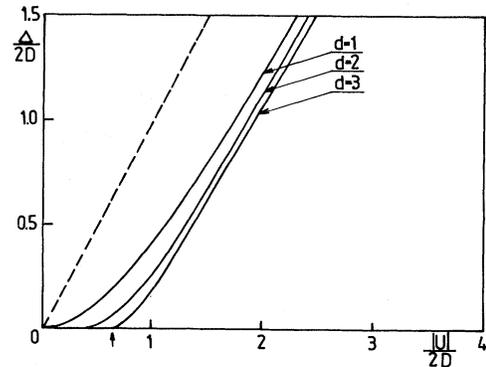
FIG. 21. Binding energies of the on-site pairs in the  $U < 0$  Hubbard model for different dimensionalities: dashed line, asymptotics for  $|U| \rightarrow \infty$  ( $\Delta = |U|$ ). A square lattice is assumed for the 2D results and a simple cubic lattice, for the 3D results.
