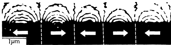
FIG. 42. Ten-times amplified interference micrograph of recorded cobalt magnetic tape (bit length, 0.15 \mu\text{m} ). Only leakage fluxes can be observed.
