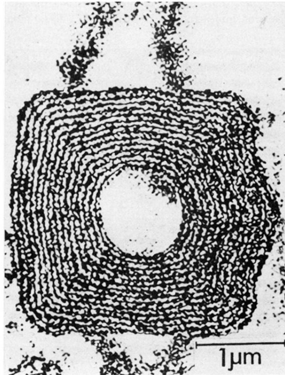
FIG. 46. Two-times amplified interference micrograph of toroidal magnet. Since contour fringes indicate magnetic flux in h/2e units, only \frac{1}{15} of the total flux, i.e., a flux of h/2e is leaking outside the toroidal, which is too small to explain the observed phase shift in Fig. 45(b).
