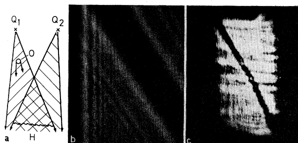
FIG. 22. Image reconstruction of thin tungsten filament (Möllenstedt and Wahl, 1968): (a) schematic for hologram formation; (b) electron hologram; (c) reconstructed image. An optical image was reconstructed from an off-axis one-dimensional electron hologram for the first time.
