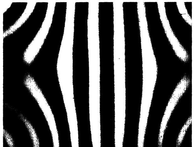
FIG. 11. A convective pattern observed using a Doppler velocimetry flow visualization technique with computer enhancement (Gollub and Heutmacher, 1984).
