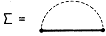
FIG. 3. Truncated Dyson equation for the self-energy part. The dashed line and dots denote the potential V in the BCS case, or the photon propagator and emission and absorption vertices in the JBW model case. The heavy line denotes a full electron propagator G=(G_0^{-1}-\Sigma)^{-1} , giving a nonlinear integral equation (the gap equation) for \Sigma .
