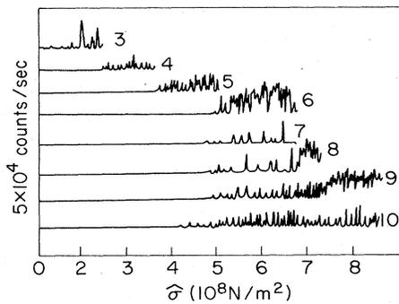
FIG. 39. Intensity of acoustic emission from Nb-Ti wire as a function of stress after several loading cycles (Pasztor and Schmidt, 1978).
