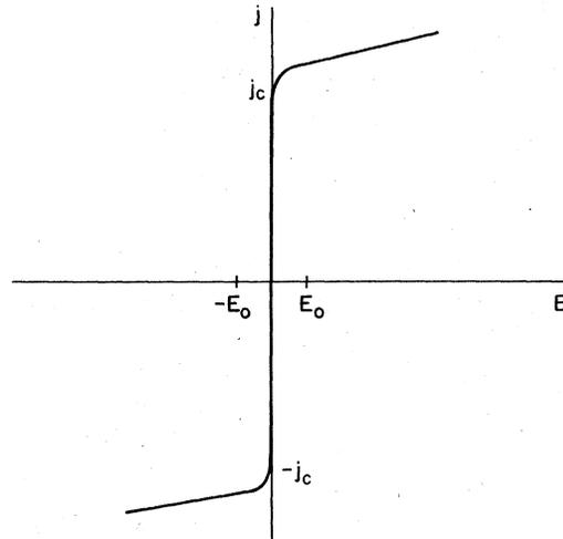
FIG. 2. Current-voltage characteristic of a hard superconductor.
