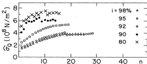
FIG. 36. Maximum applied stress  $\hat{\sigma}_Q$  at different values of  $I/I_c$  as a function of the number of on-off cycles for a superconducting composite (Pasztor and Schmidt, 1978). The sample was under vacuum.
