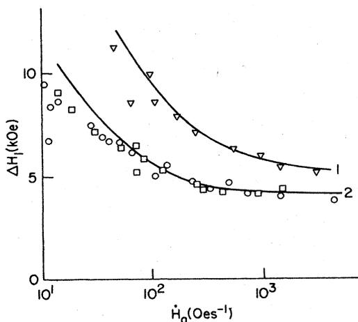
FIG. 19. Experimental data from Wipf and Lubell, 1965 (symbols) and theory (solid lines): Curve 1 and  $\nabla$ ,  $T_0 = 4.2 \text{ K}$ ; curve 2 and  $\circ$ ,  $\square$ , two different samples at  $T_0 = 2.5 \text{ K}$ .
