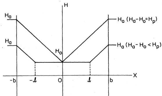
FIG. 5. Magnetic field distribution in a plane plate.
