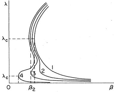
FIG. 33. Evolution of  $\lambda(\beta)$  curves with a variation of  $\alpha_T$  ( $w > 0$ ),  $\tau > \tau_c(i)$ : curve 1,  $\alpha_T = 0$ ; curve 2,  $\alpha_T < \alpha_2$ ; curve 3,  $\alpha_T = \alpha_2$ ; curve 4,  $\alpha_T > \alpha_2$ .
