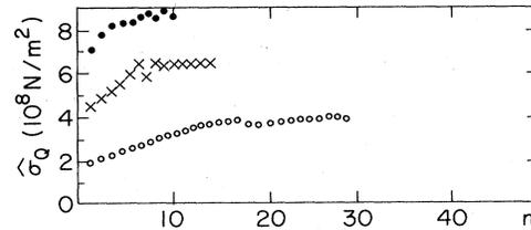
FIG. 37. The value of  $\hat{\sigma}_Q(n)$  for a superconducting composite under different conditions of external cooling,  $I/I_c = 95\%$ :  $\bullet$ , sample placed in liquid helium;  $\circ$ , sample under vacuum;  $\times$ , heat-insulated sample in liquid helium (Pasztor and Schmidt, 1978).
