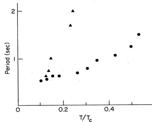
FIG. 26. Experimentally measured period of oscillations in Nb-Zr (▲) and Nb (●) samples as a function of temperature (Zebouni *et al.*, 1964).
