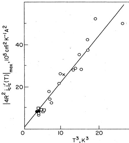
FIG. 23. The value of  $(4R^2 j_c' / \partial T)_{\max}$  as a function of  $T^3$  (Lange and Verges, 1974). Theory and experimental data for different samples.
