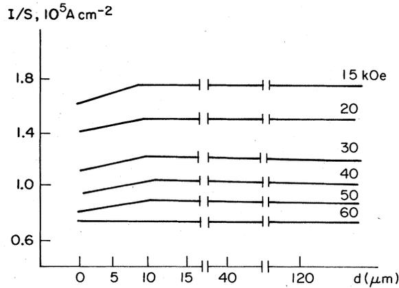
FIG. 24. Dependence of transport current in the wire upon thickness of normal cladding (Lazarev and Goridov, 1972).
