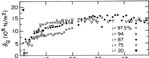
FIG. 35. Dependence of  $\hat{\sigma}_Q$  upon  $n$  for a liquid-helium-cooled Nb-Ti wire, at different values of the  $I/I_c$  ratio (Pasztor and Schmidt, 1978).
