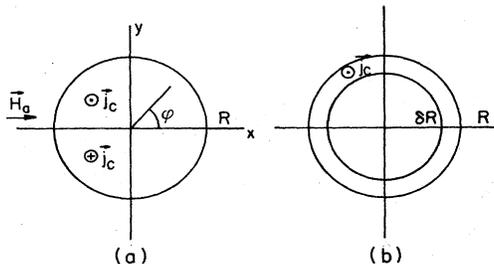
FIG. 10. Cylindrical samples: (a) wire in a transverse external magnetic field  $H_a > H_p$ ,  $I=0$ ; (b) wire with preset transport current.
