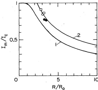
FIG. 11. Maximum transport current in the wire as a function of the ratio  $R/R_0$ : Curve 1, uncoated wire; curve 2, wire clad with normal metal to a thickness of  $d > d_c$ . The points show experimental data from Lange and Verges (1974).
