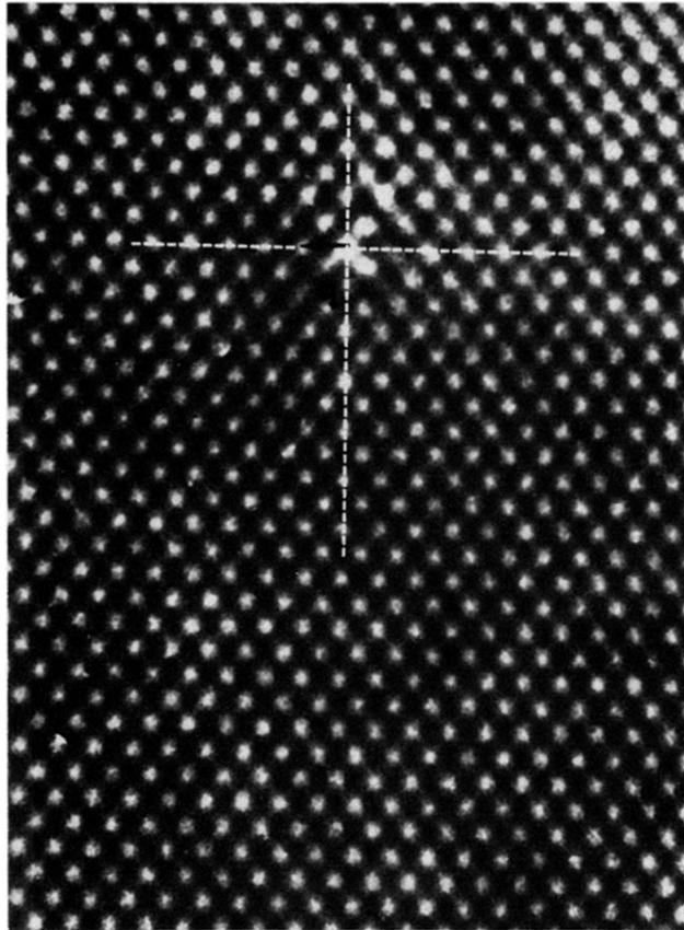
FIG. 9. Dislocation in a germanium crystal. This electron microscope photograph has been obtained by A. Bourret (CENG, Grenoble). The plane of the picture is perpendicular to the  $110$  axis; the Burgers vector of the dislocation is  $1\bar{1}0$ .
