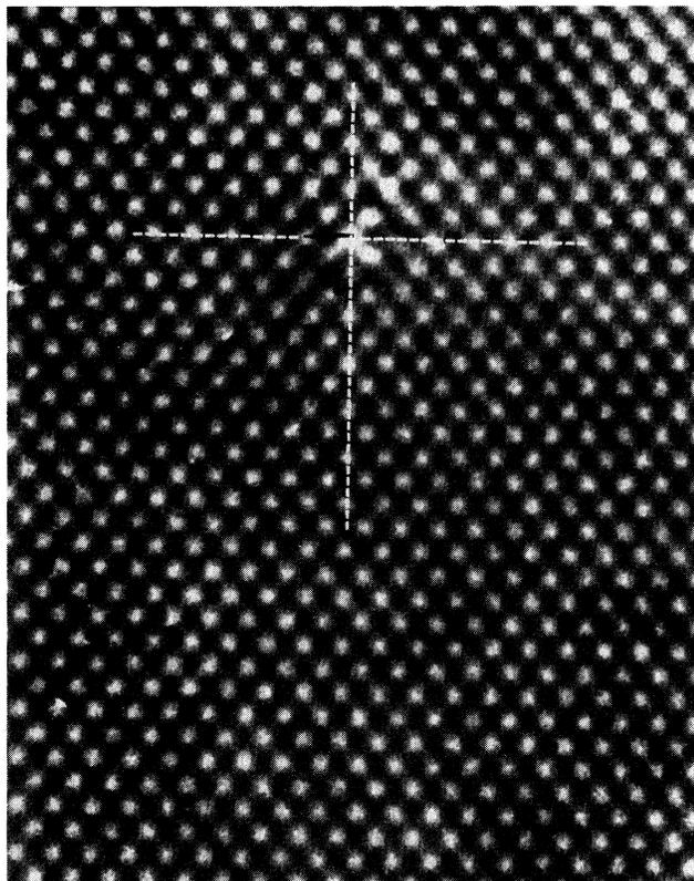
FIG. 9. Dislocation in a germanium crystal. This electron microscope photograph has been obtained by A. Bourret (CENG, Grenoble). The plane of the picture is perpendicular to the 110 axis; the Burgers vector of the dislocation is  $110$ .
