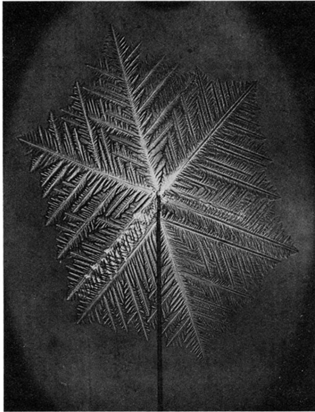
FIG. 3. Photograph of dendritic ice crystal grown in pure water at an undercooling of T_M - T = 2.34^\circ\text{C} (Fujioka, 1978).
