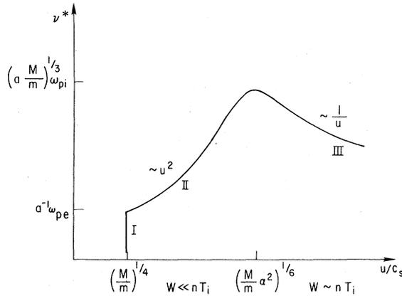
FIG. 2. Schematic drawing of the anomalous collision frequency  $\nu^*$  for ion acoustic turbulence as a function of normalized drift velocity  $u/c_s$ .
