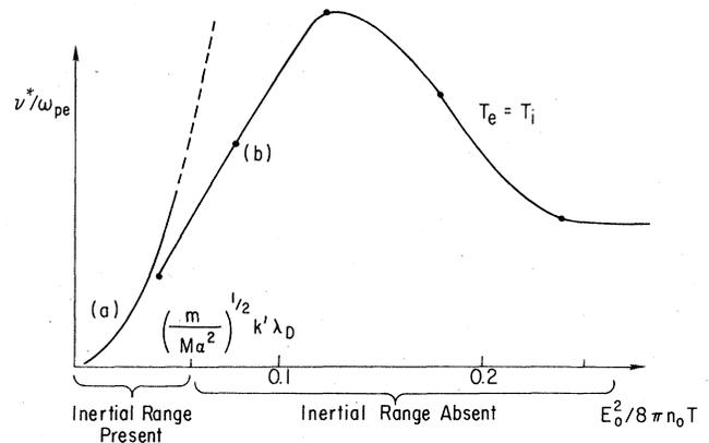
FIG. 4. Anomalous collision frequency  $\nu^*$  as a function of pump field  $E_0$  in the regime of modulational instability. (a) Theoretical scaling from inertial range arguments (see text). (b) Empirical dependence from numerical simulations (Kruer *et al.*, 1970).
