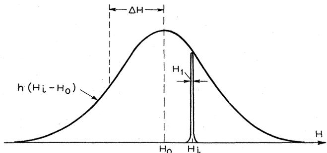
FIG. 13. "Spin packets" and spectral diffusion.
