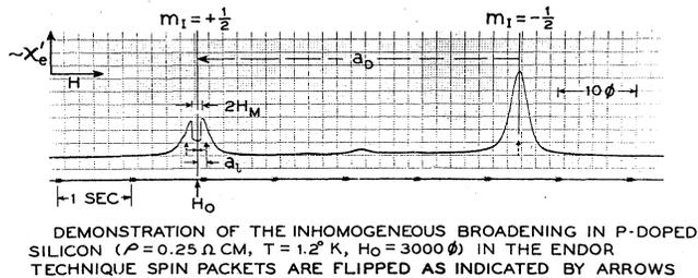
DEMONSTRATION OF THE INHOMOGENEOUS BROADENING IN P-DOPED SILICON ( $\rho = 0.25 \Omega \text{ CM}$ , T=1.2° K,  $H_0 = 3000 \phi$ ) IN THE ENDOR TECHNIQUE SPIN PACKETS ARE IDENTIFIED AS INDICATED BY ARROWS
