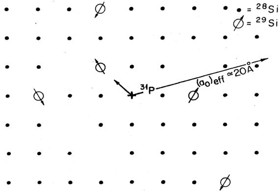
FIG. 9. Donor wave functions in Si and <sup>29</sup>Si nuclei: schematic.
