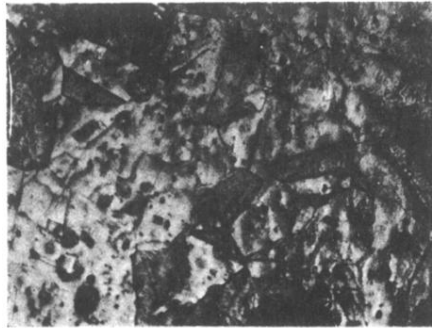
FIG. 8. Same as Fig. 7. Etched to show the outlines of the copper crystal grains, \times 200 .
