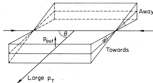
FIG. 11. Schematic description of the kinematical regions used in the study of large  $p_T$  events.
