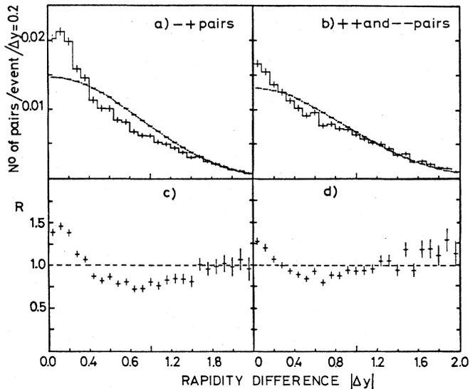
FIG. 29. The distribution of rapidity difference of pairs of particles in the away region (full line). Also shown is the equivalent distribution for uncorrelated pairs. (c) and (d) show normalized rapidity difference distributions obtained by taking the ratio of the distributions of (a) and (b), respectively, to the background distributions of these figures (Della Negra *et al.*, 1976b).
