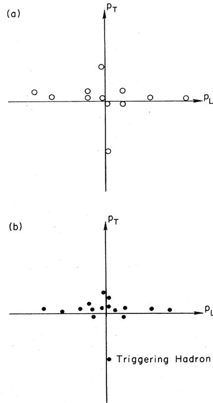
FIG. 38. Pictorial representation of the distorted momentum space distribution of (a) the constituents immediately after the hard scattering (open circles) and (b) the final hadrons (full dots) resulting from the trigger bias coupled with the  $p_T$  distribution of the constituents in the initial hadrons.
