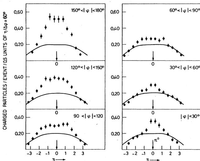
FIG. 12. Charged particle densities for the  $\pi^0$  trigger at  $90^\circ$  data, averaged over events with  $p_T$  of the  $\pi^0 > 2$  GeV/c. The solid lines give charged-particle densities in minimum bias triggers (Eggert *et al.*, 1975a).
