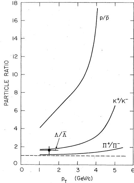
FIG. 7. Particle-antiparticle ratios for 300 GeV  $p$ - $p$  collisions extracted from Chicago-Princeton data (Antreasyan *et al.*, 1977a, 1977b).  $\Lambda/\bar{\Lambda}$  point from (Büsser *et al.*, 1976b).
