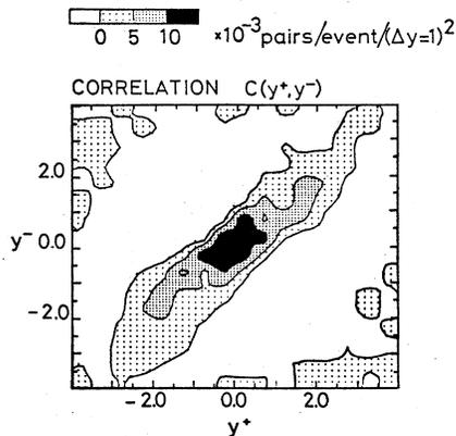
FIG. 30. Contour lines for the correlation function  $C(y_1, y_2) = \rho^2(y_1, y_2) - \rho^1(y_1)\rho^1(y_2)$  for particle pairs of opposite charge in the away region.  $\rho^2$  and  $\rho^1$  denote two- and one-particle density distributions, respectively (Della Negra *et al.*, 1976b).
