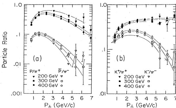
FIG. 6. The particle ratios versus  $p_T$  for 200, 300, and 400 GeV  $p$ - $p$  collisions (Antreasyan *et al.*, 1977b).
