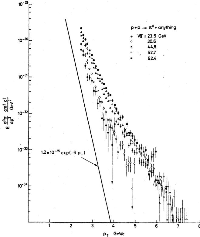
FIG. 1. Invariant cross section for  $\pi^0$  production at  $90^\circ$  for five center-of-mass energies. The extrapolation from data with  $p_T < 1$  GeV/c is shown for comparison (Büsser *et al.* 1976a).
