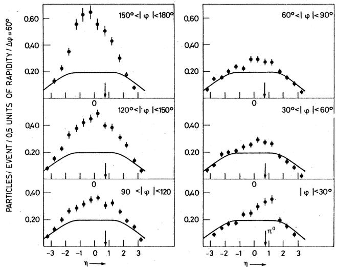
FIG. 27. Charged-particle densities for the  $\pi^0$  trigger at  $53^\circ$ . The solid lines give charged-particle densities for minimum bias trigger (Eggert *et al.*, 1975a).
