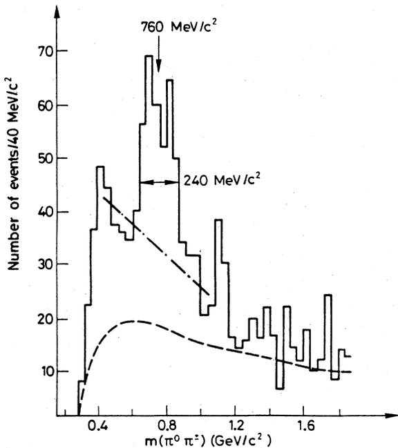
FIG. 21. The  $\pi^0\pi^+$  mass distribution in the towards region for large  $p_T\pi^0$  events. The dashed line is the mass distribution for uncorrelated particles and the dashed-dotted line represents assumed background (Darriulat *et al.*, 1976).
