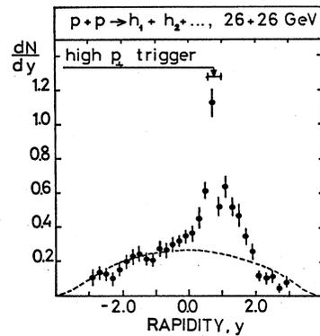
FIG. 18. The rapidity distribution of negative secondaries in the towards region for the events with  $45^\circ$  positive particle with  $p_T > 2$  GeV/c. The full line represents the equivalent distribution for normal events (Della Negra *et al.*, 1976b).
