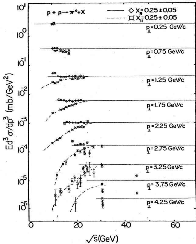
FIG. 4. The  $\pi^0$  invariant cross section  $E(d^3\sigma/dp^3)$  for constant  $x_R$  or  $x_{\parallel}$  and constant values of  $p_T$  vs  $\sqrt{s}$  (Taylor *et al.*, 1976).
