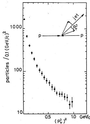
FIG. 19. The transverse momentum squared distribution with respect to the jet axis of particles forming the jet (Della Negra *et al.*, 1976b).
