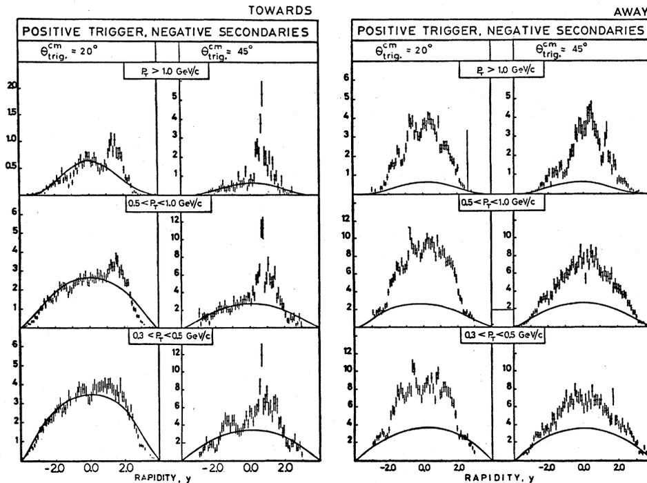
FIG. 14. Rapidity distribution of negative secondaries in the *a* "towards" azimuthal angle and *b* "away" azimuthal angle for the  $20^\circ$  and  $45^\circ$  positive triggers. Full line indicates the respective distribution of normal events. The vertical scale is the charged multiplicity, times 100, per interval of  $\Delta\phi$  and  $\Delta y$  (in  $\text{radian}^{-1}$ ) (Della Negra *et al.*, 1976a).
