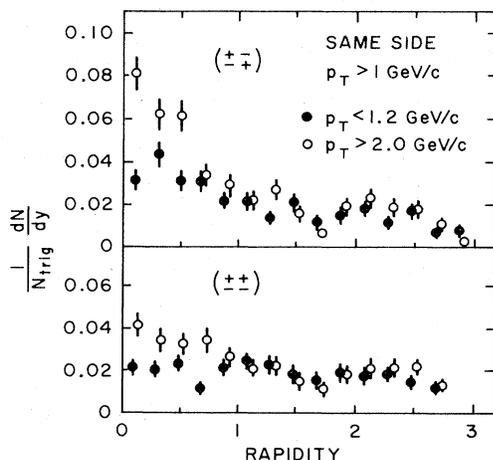
FIG. 24. Rapidity distribution of secondaries with  $p_T > 1 \text{ GeV}/c$  in the events with large  $p_T$  trigger at  $y=0$ .  $P_w$  is the  $p_T$  of the trigger (Møller, 1976).
