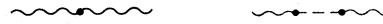
FIG. 4. These diagrams represent the leading corrections to the free photon propagator in the Higgs theory. The wavy line is the photon, and the dashed line is the \phi'(0) . The vertex in Fig. 4(a) is given by e_0^2(\eta^2/2) , while each vertex in Fig. 4(b) is given by iq_\mu(\eta e_0/\sqrt{2}) , where q_\mu is the “photon” four-momentum.
