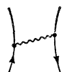
FIG. 18. Contribution of a virtual zero-sound excitation (shown by the wiggly line) to the effective particle-hole interaction.
