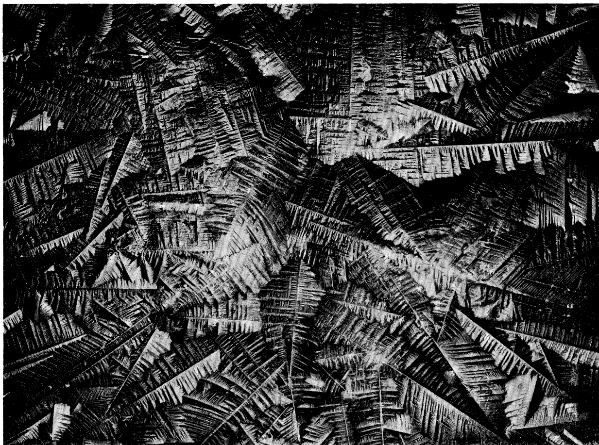
FIG. 10. The surface of an ingot of antimony showing dendritic crystals which have growth interference with each other. (This pattern was the mystic Star of Antimony of the alchemists.) About \frac{2}{3} natural size. (Courtesy The Science Museum, London.)
